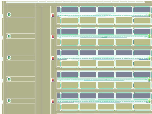
Figure 4: Channels drawn in a 150 L/s are extremely wide and are causing the flocculation hopper to be extremely wide.
