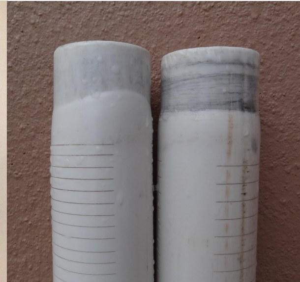
Figure 3: Molded OStaRS Pipe Ends
