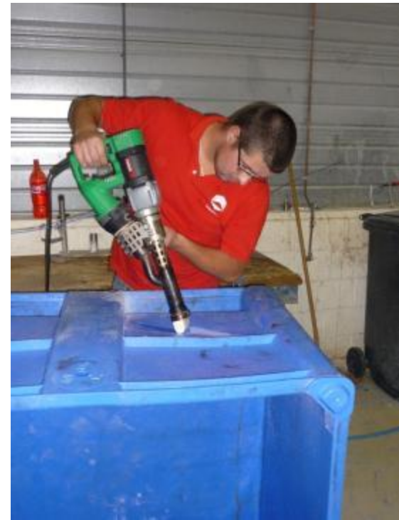
Plastic box repair Netherlands (Polyethylene)
