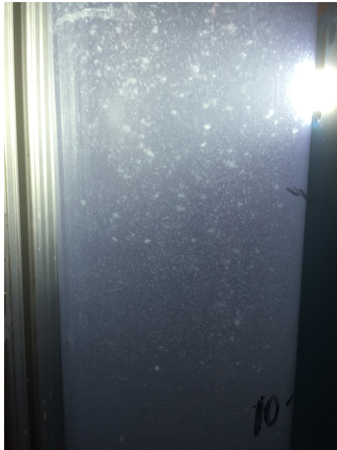
Figure 11: Floccs passing through the PVC pipe sedimentation tube are large enough to see with the naked eye, thus proving that the flocculator design equations are valid for high flow rates.
