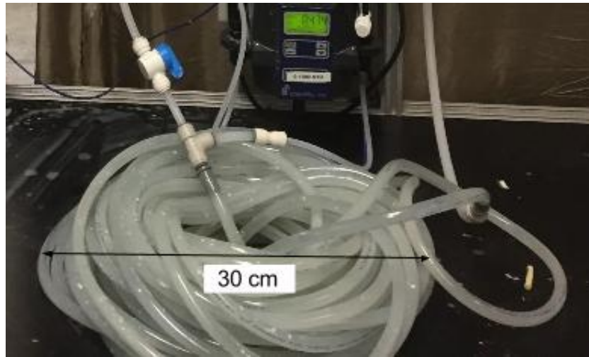
Figure 5: The Fall 2015 High Rate Sedimentation team used a tube flocculator that was made with 0.95 cm (3/8 in) flexible tubing and coiled into a 30 cm diameter circle.
