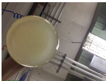
Figure 12: Bottom layer of sample with 1 g of gelatin
