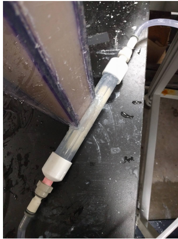
Figure 4: Top view of the inlet after being glued to the tank.
