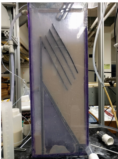
Figure 11: The floc blanket that formed in the sedimentation tank at an upflow velocity of 3mm/s with plate settlers in the top part of the tank
