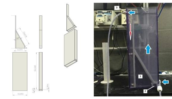
Tank with the insert (1) and jet reverser (2) and outlet (3). Blue arrows show water entering, rising through the tank and exiting, the red arrow points into the sludge hopper where flocs will fall and consolidate.
