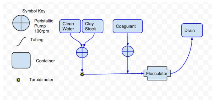
Figure 4: Schematic of Initial Testing Apparatus. This is meant to mimic the rapid mix pipe and flocculator of the AguaClara plant. The flocculator is detachable and is weighed before and after testing to determine weight of coagulant build-up.
