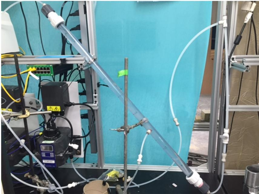
Figure 10: This figure shows the tube settler constructed by the team. After water flows through the flocculator, it enters the tube settler through the inlet (about a third of the way up) and flocs settle out and clean water exits the top of the tube.
