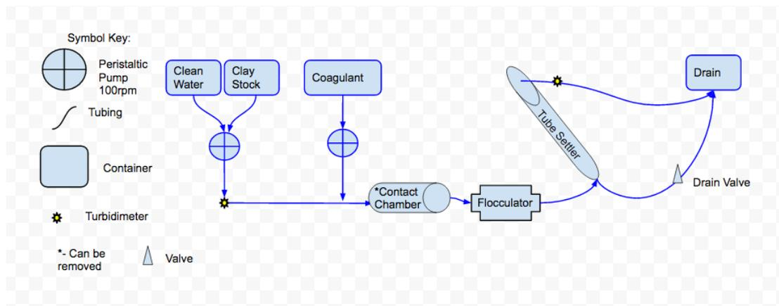
Figure 3: Schematic of Final Testing Apparatus. This is meant to mimic the rapid mix pipe and flocculator of the AguaClara plant. The contact chamber is detachable and new ones can be attached for different tests.
