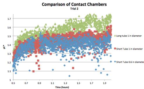
Figure 20: This graph is the second trial of a test that compared the three contact chambers built by the team. This was done to show the consistency of the data.
