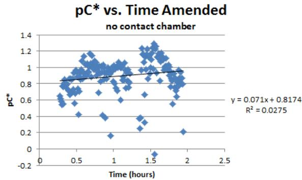
Figure 14: This figure displays the  $pC^*$  values for the first two hours of the experiment, during which time the performance of the tube settler was relatively constant.
