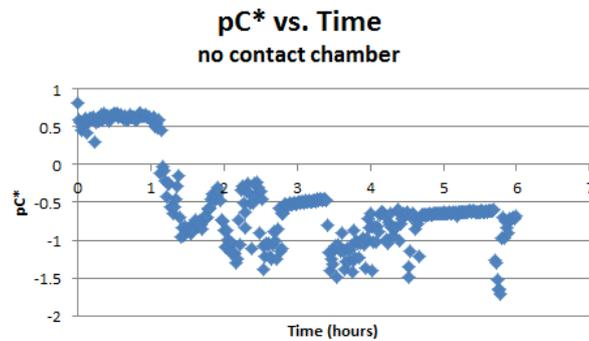
Figure 11: This figure displays the  $pC^*$  values for the first trial of the experiment with the tube settler. The experiment was run at the same initial conditions as the previous experiments: 5 NTU influent turbidity and a 2 mg/L coagulant dose. The team predicted that the tube settler hit breakthrough after one hour of the experiment.
