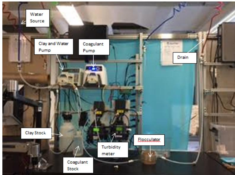
Figure 5: Initial Testing Apparatus Image. Clay and coagulant stocks are the plastic bottles in the lower left corner. Fresh water flows in the blue tube. The pumps are in the upper left hand corner of the photo, the water then flows into the turbidity meters on the bottom left hand side and then through the flocculator in the middle then out the red tube to the drain.
