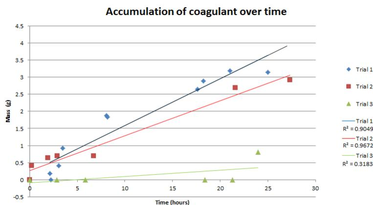
Figure 7: In these experiments the change in mass in the flocculator during a twenty-four hour test was recorded. The influent was a clay water solution with a turbidity of 5 NTU. The mass was zeroed at the beginning of the experiment so negative mass means a decline in mass.
