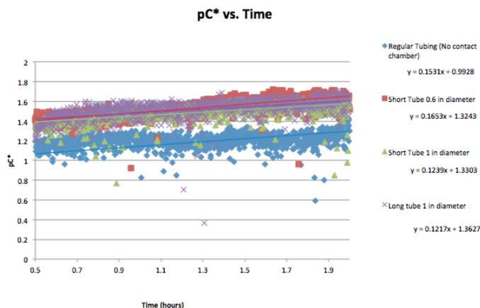
Figure 17: This graph is the first trial of a comparison of the different contact chambers built by the team. The regular tubing parameter is the control. The three contact chambers varied radius and residence time. From this the optimal contact chamber design could be inferred.
