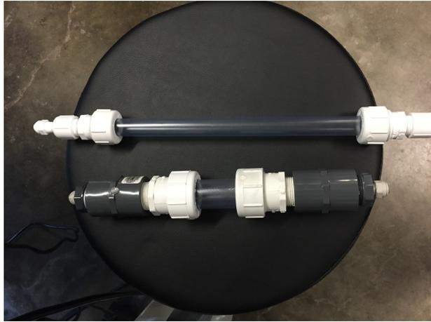
Figure 15: This figure shows the two contact chambers designed and built by the team. The residence time and volume for both were the same; however, radius differed. The contact chambers will be used to test the impact surface area of the contact chamber has on coagulant loss.
