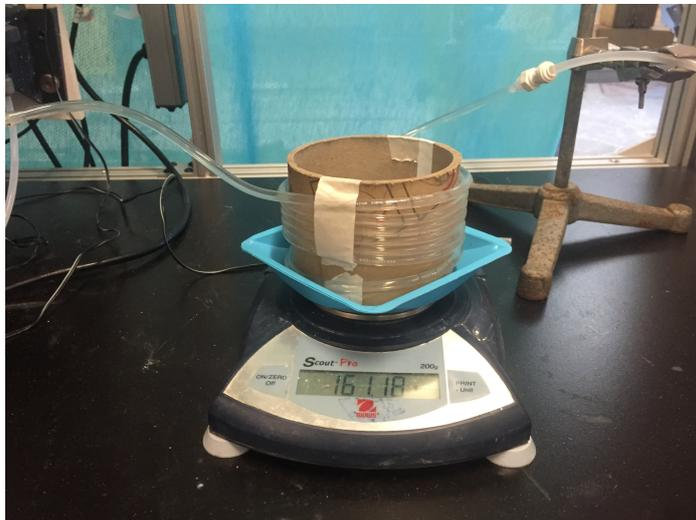
Figure 6: This photo shows the current setup of the flocculator with the mass balance. This is the setup that was used to continuously record the mass of the flocculator throughout the experiment. The change in mass represents the coagulant and clay sticking to the walls.
