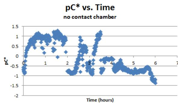
Figure 13: This figure displays the  $pC^*$  values, or the negative log of the effluent over influent turbidities. The  $pC^*$  values were measurements of the performance of the tube settler. The team observed a steady performance for approximately 2 hours, until the tube settler hit breakthrough.
