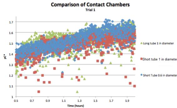
Figure 19: This graph is the first trial of a test that compared the three contact chambers built by the team. The three contact chamber differed in residence time or radius as shown on the graph. From this information the team could determine the best shape for a contact chamber.
