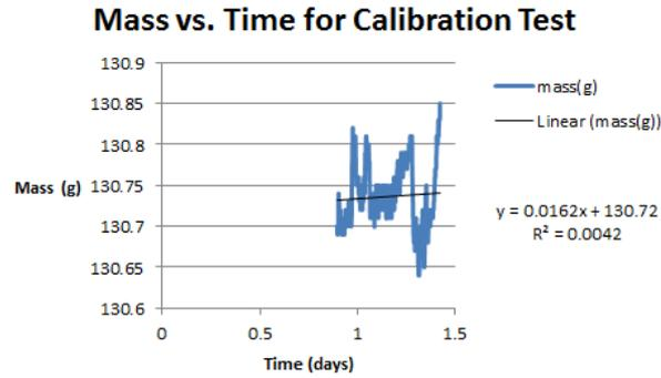
Figure 9: This figure displays the result of the calibration test, in which only water was pumped through the apparatus for 17 hours. The mass of the flocculator was relatively constant over the experiment time.
