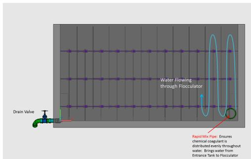
Figure 1: This figure displays the Rapid Mix Pipe and Flocculator of the AguaClara plants. Water enters through the Rapid Mix Pipe on the right-hand side and exits the system through the flocculator on the left-hand side.
