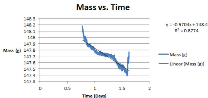
Figure 8: This figure displays the results from the first trial of the third iteration. The mass of the flocculator decreased throughout the experiment.
