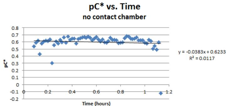
Figure 12: This figure displays the  $pC^*$  values for only the first hour of the experiment, during which time the performance of the tube settler was relatively constant, as can be seen by the zero-sloped graph.
