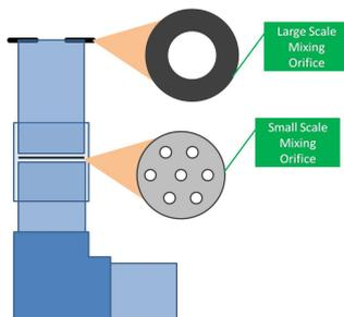
Figure 2: This figure displays the designs of small and large scale mixing in the Rapid Mix Pipe.
