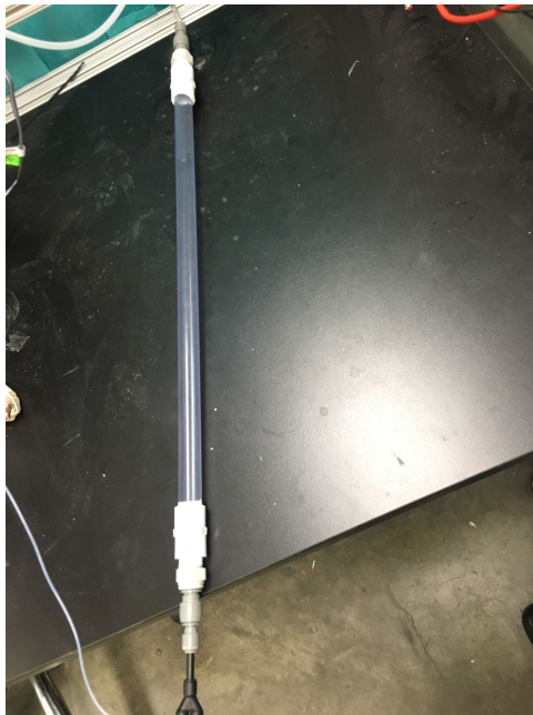
Figure 7: The rapid mix chamber. It has a length of 0.5 meters and 0.52 inches. When used, it is after the coagulant is injected into the system's water flow. The solution then enters the chamber through a 1/16 in orifice through a push-to-connect connector.
