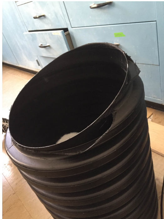
Figure 4: The cut was made at a 15° angle. When pieced together with the other section of pipe, the two will form a 30° bend.
