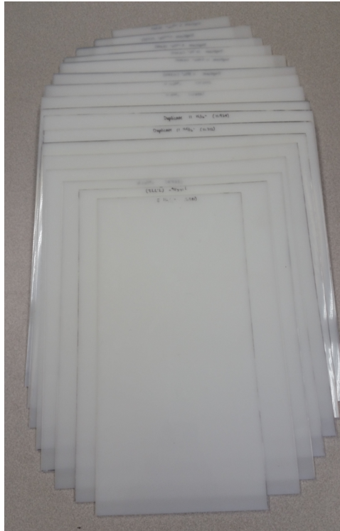
Figure 9: All 17 HDPE plate settlers before assembly into the bundle. Widths vary from 12" to 5.901".
