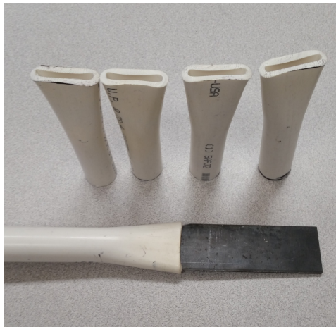
Figure 13: Finished jet diffusers and diffuser on metal mold.
