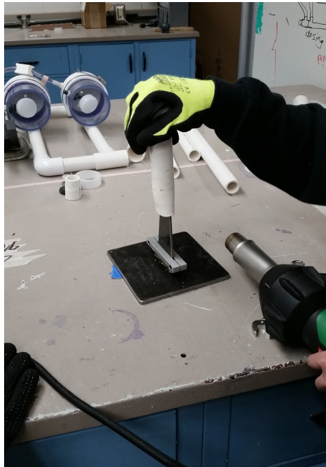
Figure 12: Molding the jet diffusers using the plastic welder and the metal mold.
