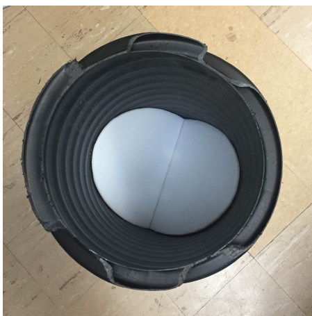
Figure 7: The base is comprised of two semi-ellipse pieces, welded together along their major axis. The slopes of these sheets measure 60^\circ . The jet reverser is not present in the photo.
