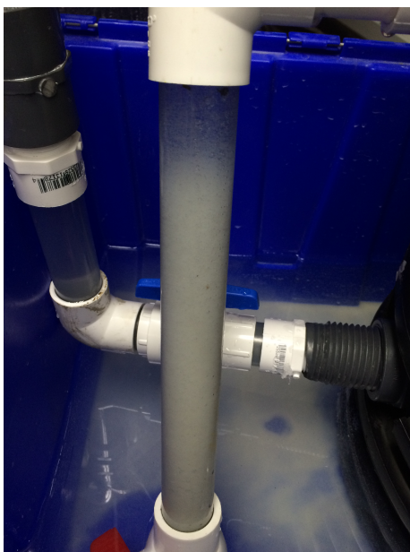
Figure 17: After priming, the flocs captured by the floc hopper are visible.
