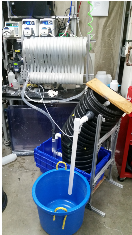
Figure 15: Turbid water was run through the tank at the target flow rate for 8 hours.
