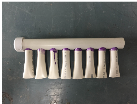
Figure 14: The diffusers were fastened to the inlet manifold with a coat of PVC primer and glue.
