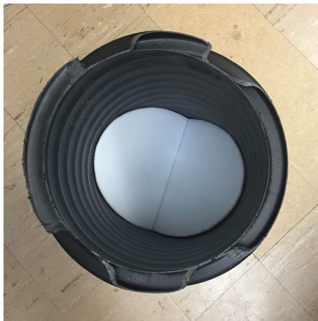
Figure 6: The base is comprised of two semi-ellipse pieces, welded together along their major axis. The slopes of these sheets measure 60^\circ . The jet reverser is not present in the photo.
