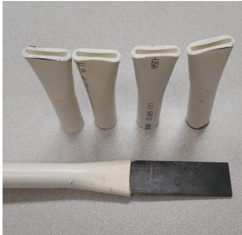
Figure 12: Finished jet diffusers and diffuser on metal mold.
