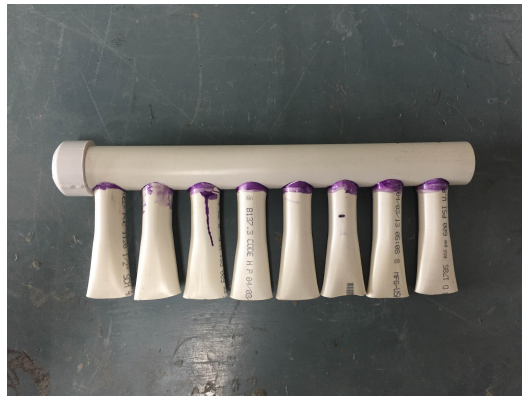
Figure 13: The diffusers were fastened to the inlet manifold with a coat of PVC primer and glue.
