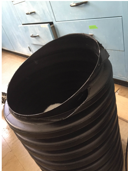
Figure 3: The cut was made at a 15^\circ angle. When pieced together with the other section of pipe, the two will form a 30^\circ bend.
