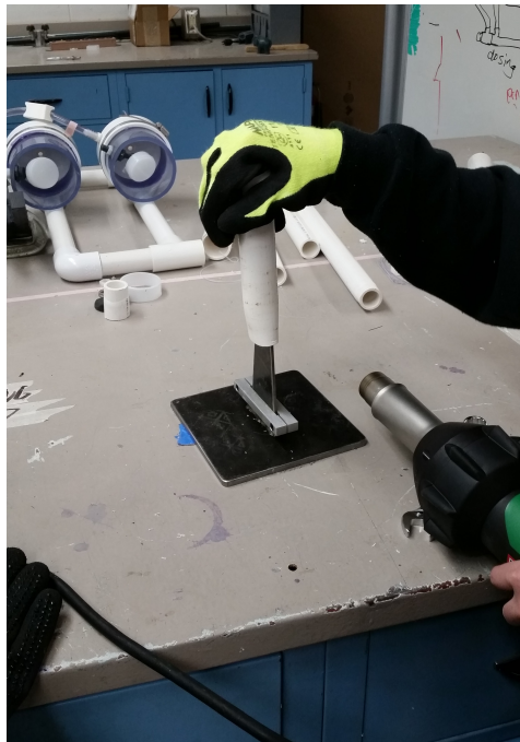
Figure 11: Molding the jet diffusers using the plastic welder and the metal mold.
