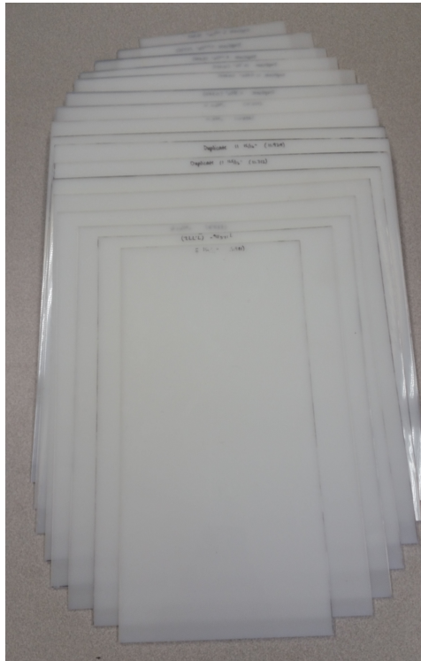
Figure 8: All 17 HDPE plate settlers before assembly into the bundle. Widths vary from 12" to 5.901".
