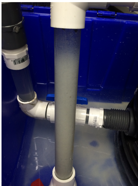
Figure 16: After priming, the amount of flocs captured by the floc hopper are visible.
