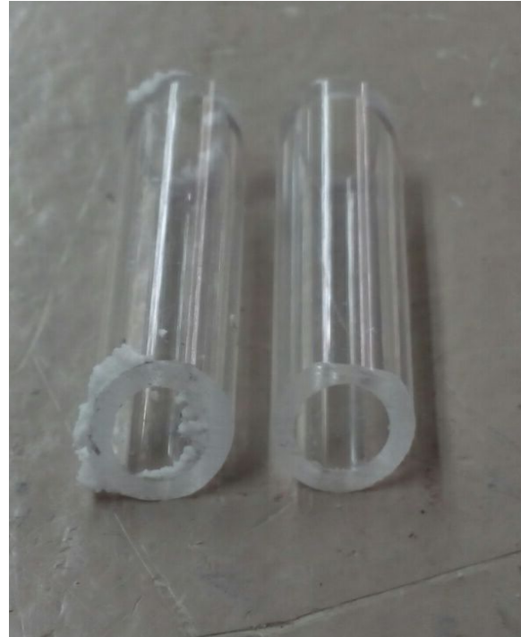
Before - After of cleaning spacers
