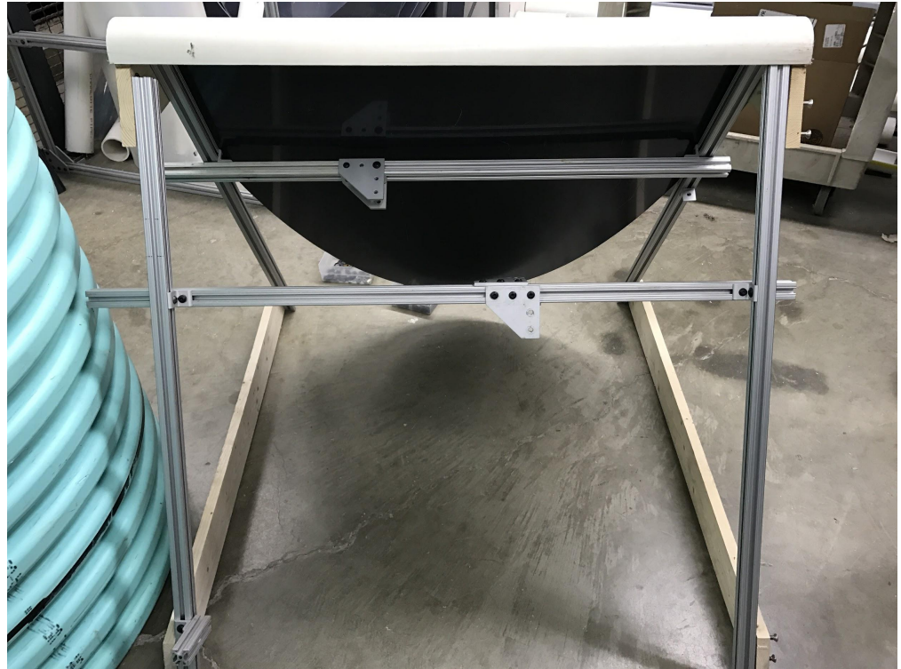
The jig used to hold the half ellipses to the jet reverser at the correct angle
