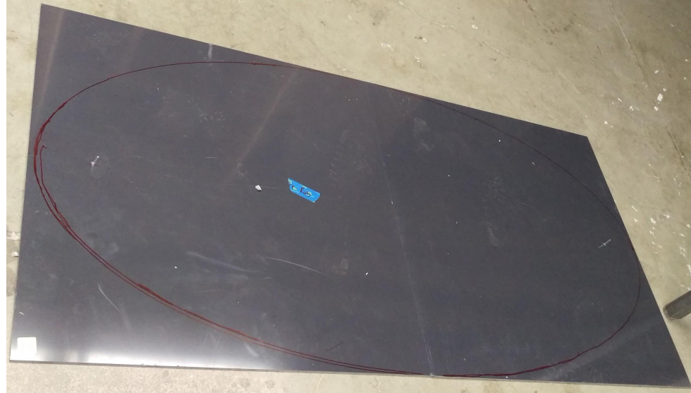
The pvc plates after having the ellipse circumference drawn
