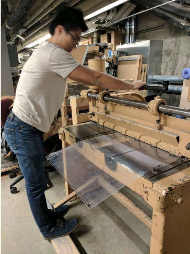
Using the shear to cut the plate settlers
