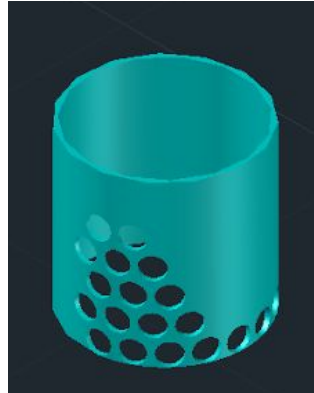
Figure 6: AutoCAD output of LFOM
