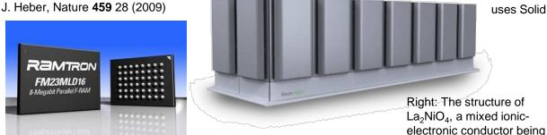
A ferroelectric random access memory chip from Ramtron (and Texas Instruments, below)
