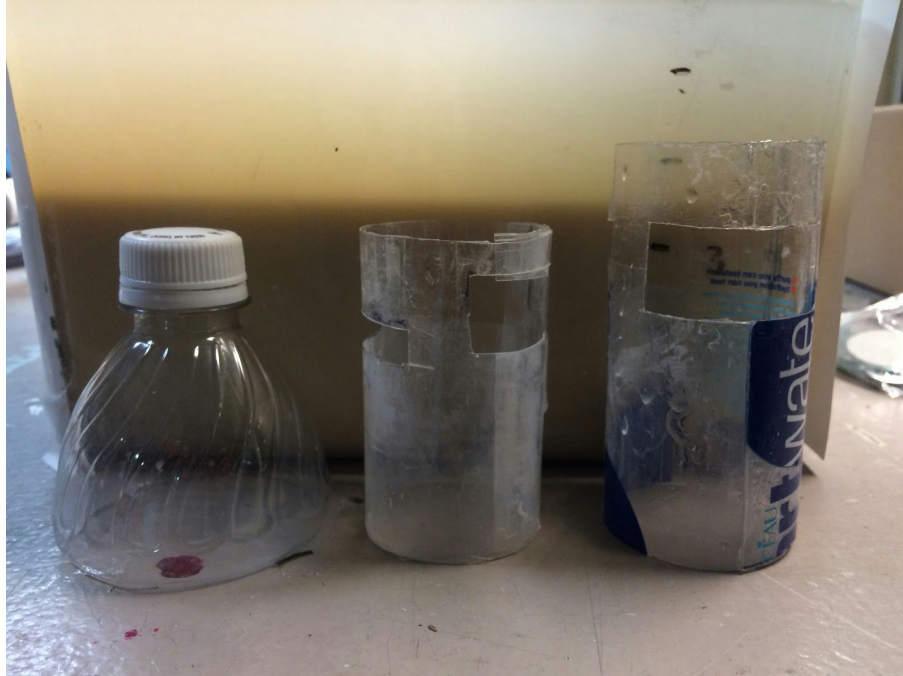
Figure 8: Progression of probe tips to condense floccs (from left to right)
