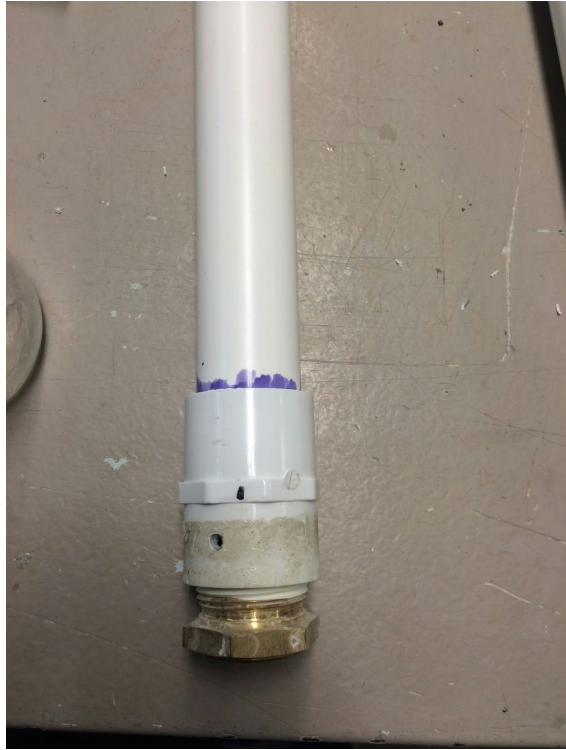
Figure 3: Probe with PVC Cover, Light Source and Plastic Cylinder Removed (Exposing Lens)
