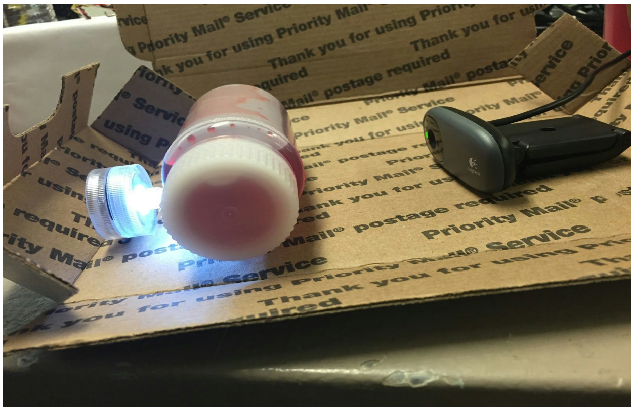
Figure 2: Crude Spectrophotometer Model
