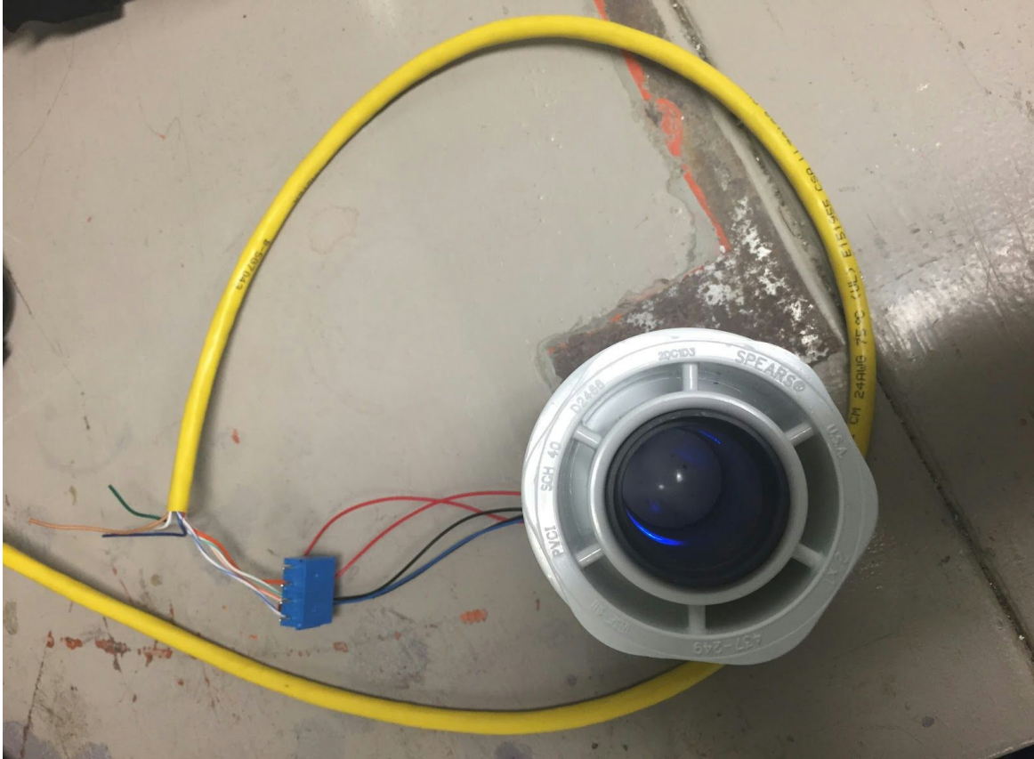
Figure 5: Ambient Light Photosensor (Top-view)
