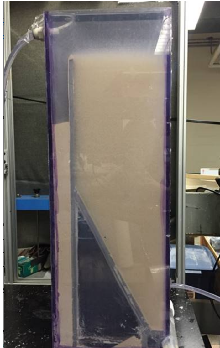
Figure 1: The floc blanket reached the top of the floc weir and then wasted into the floc hopper, as seen on the lefthand side of the apparatus. The jet reverser can be seen in the bottom righthand corner of the apparatus (Anyene et al., 2016)
