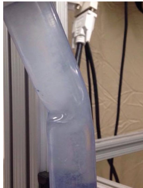
Figure 16: The model with a dimpled bend.
