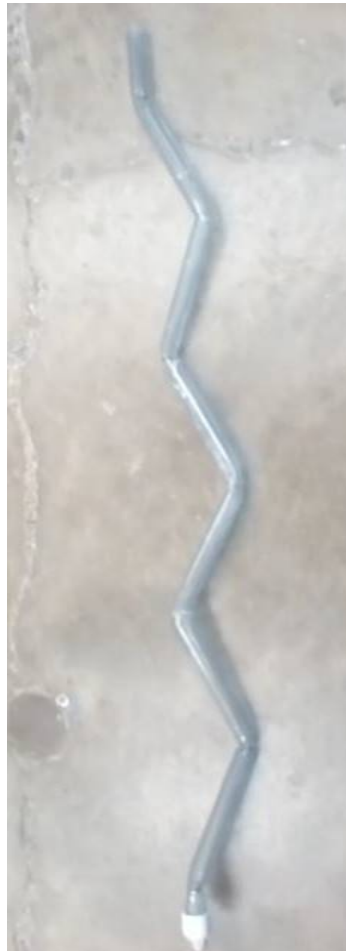
Figure 12: The zigzag recirculator produced lower effluent turbidity than the straight recirculator, but higher effluent turbidity than the trapezoidal recirculator.
