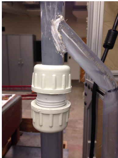
Figure 7: The compression fitting provides a removable, waterproof connection between the recirculator and the flocc weir, allowing different recirculator pieces to easily be swapped in and out.
