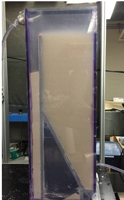
Figure 1: The floc blanket reached the top of the floc weir and then wasted into the floc hopper, as seen on the lefthand side of the apparatus. The jet reverser can be seen in the bottom righthand corner of the apparatus (Anyene et al., 2016)
