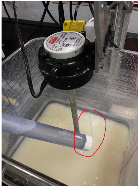
Figure 4: A short piece of pipe ensures the small clay tube will remain submerged.
