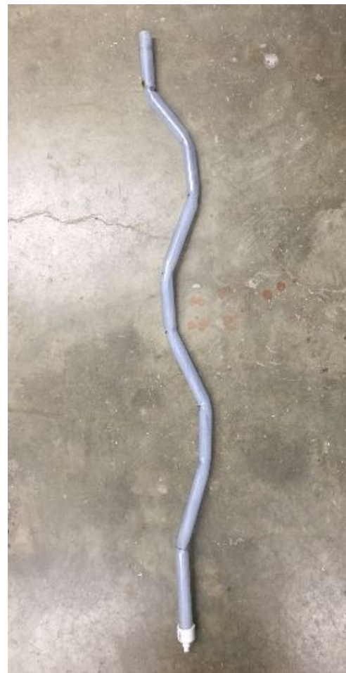
Figure 3: The trapezoidal recirculator outperformed both the straight and zigzag recirculators, raising more questions on floc blanket formation at, and below, pinch puddles.
