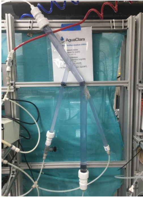
Figure 18: The general setup for the addition of a second weir at the top of the recirculator. The Fall 2017 team includes this addition in hopes that the floc blanket will stabilize and performance will stop deteriorating over time.
