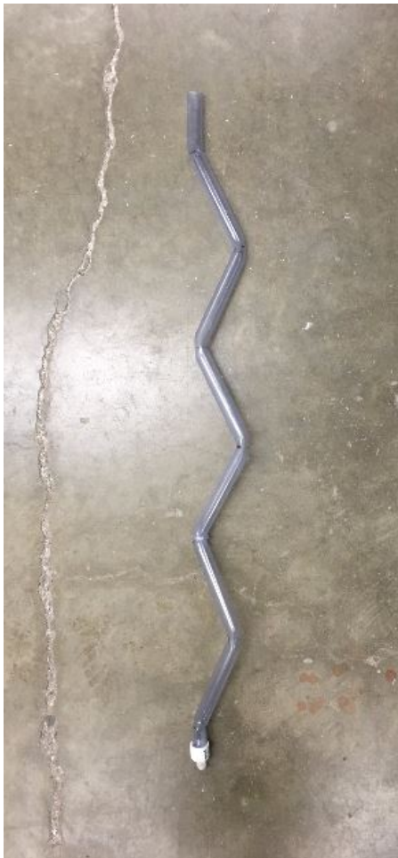
Figure 2: The zigzag recirculator produced lower effluent turbidity than the straight recirculator, but higher effluent turbidity than the trapezoidal recirculator.
