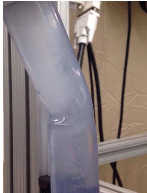
Figure 8: The model with a dimpled bend.
