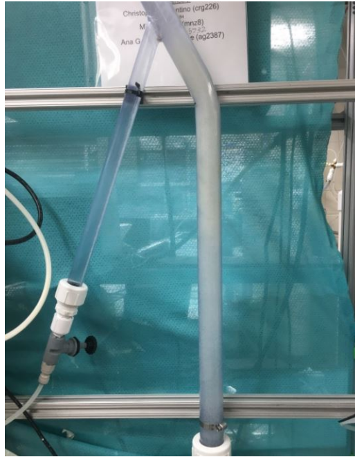
Figure 16: As the Standard Design experiment progressed, the floc blanket dissipated from the bottom up.
