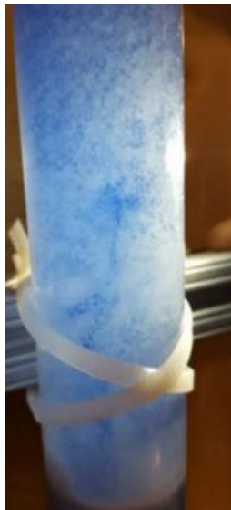
(a) The initial result after introducing the reactor with the dye feedstock. The blue dye was concentrated within the floc blanket.
