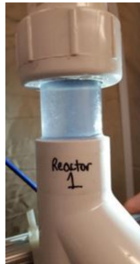
(b) While the initial result in Figure 5a was occurring within the floc blanket, the top part of Reactor 1 remained relatively clear of blue dye.
