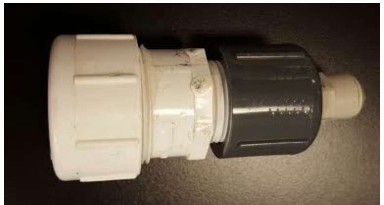
Figure 7: A close up of the pressure cap
