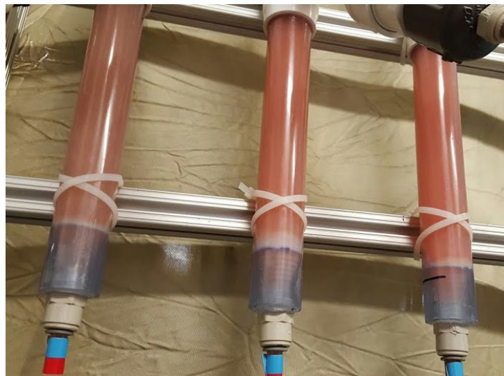
Figure 14: The diffusion of the red dye spread throughout the entire reactor. Thus, the results of floc formation and removal were inconclusive.
