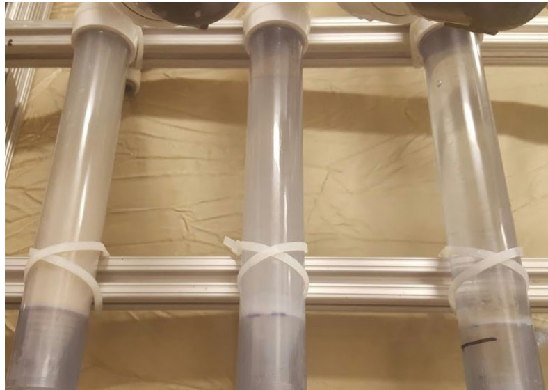
Figure 20: An early attempt of forming floc blankets. Due to the low upflow velocity, heavy sedimentation in reactor 3 was observed.
