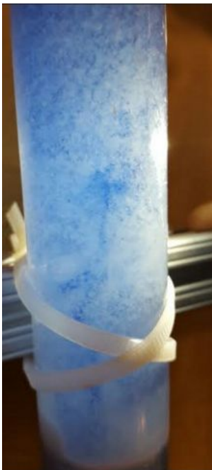
Figure 15 (Left): The initial result after introducing the reactor with the dye feedstock. The blue dye was concentrated within the floc blanket
