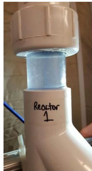
Figure 16 (Right): While the initial result in Figure 15 was occurring within the floc blanket, the top part of Reactor 1 remained relatively clear blue dye.
