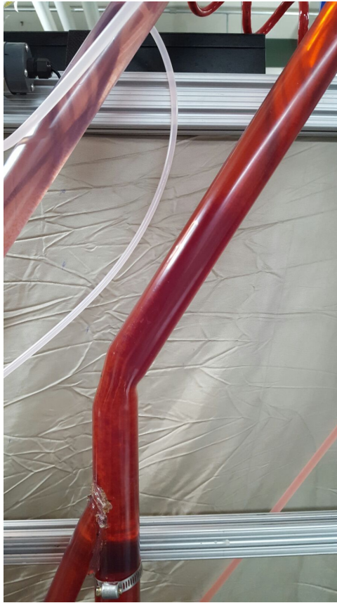
Figure 13: Accumulation of flocs in settler tube of first reactor (1.5mm/s upflow velocity).
