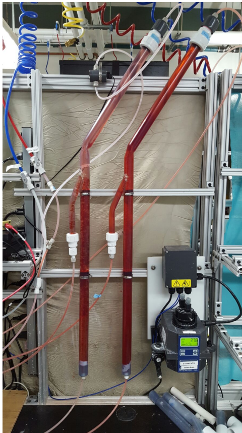
Figure 19: Sludge formation in first reactor settler tube (1.5 mm/s upflow velocity).
