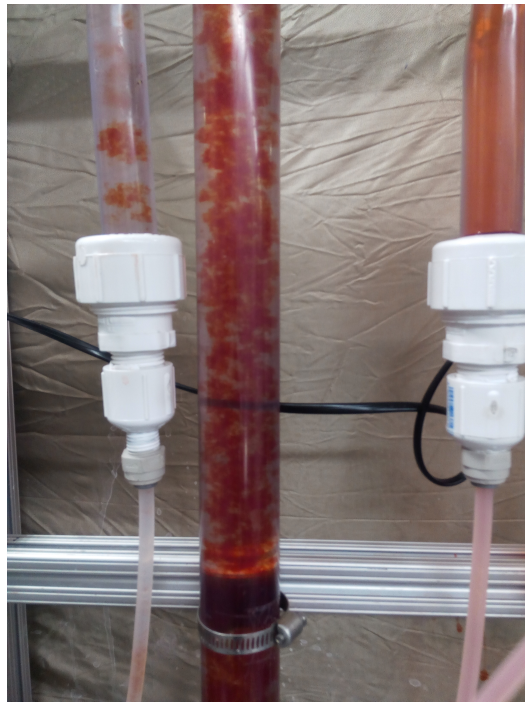
Figure 12: Floc blanket formation all along the second reactor (1.5mm/s upflow velocity).
