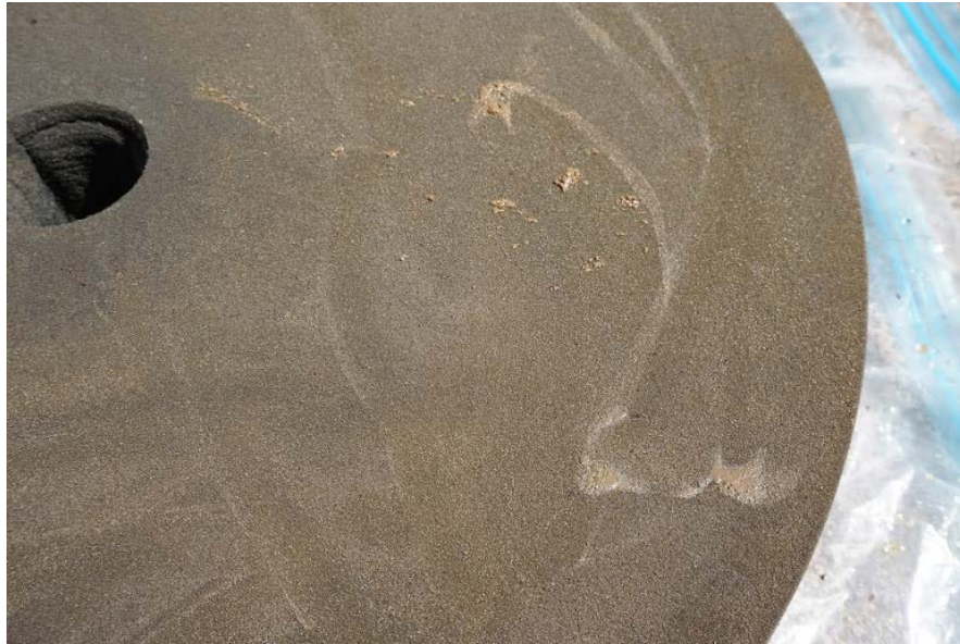
Figure 2: The bottom of most 90 ppi foam discs after five backwash cycles.
