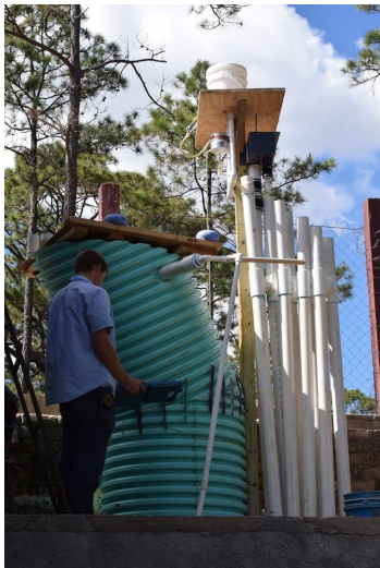
Figure 4. Field testing of the AguaClara 1 L/s drinking water treatment plant. Many of the reactor design and fabrication techniques used for this drinking water treatment plant may be used to advance the design of prefabricated UASB reactors.
