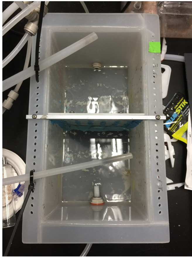
Figure 8: Effluent collection tank of the Granule Settling Test for the Conventional Reactor (lower compartment) and the Alternative Reactor (upper compartment). By visual inspection, there was no granules collected in the collection tank or trapped in the effluent tubes
