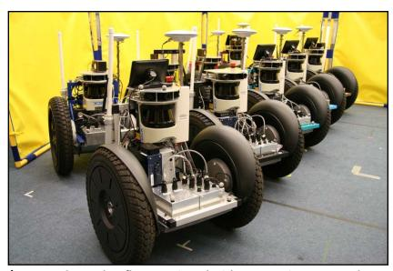
Segway RMP50/50XL outdoor robot fleet, equipped with Septentrio GPS, 180 deg FOV SICK and 270 deg FOV Hokuyo Lidar, Mimo touchscreen interfaces, Firefly Cameras, onboard IMU, mobile WiFi, custom electronics and mounting hardware.
