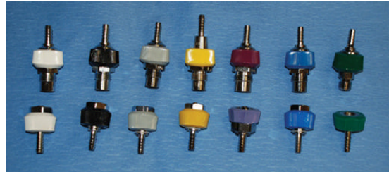
Figure 3.32 The diameter index safety system (DISS) uses a gas-specific non-interchangeable thread pattern to avoid incorrect gas delivery. Gases are also color coded as apparent in the figure. Source: Thomas Riebold, College of Veterinary Medicine, Oregon State University, Corvallis, OR, USA. Reproduced with permission of Thomas Riebold.
