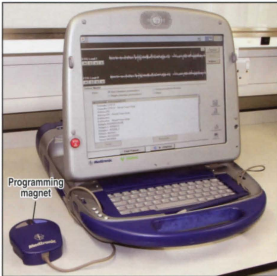
20.5 Pacemaker programmer. A foldable screen and programming magnet are features of all models.
