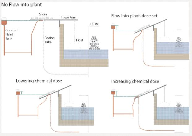
**To change** the amount of chemical that is dosed, the slider is adjusted along the lever arm. There is a slider on the lever arm for each chemical being dosed, typically two.
