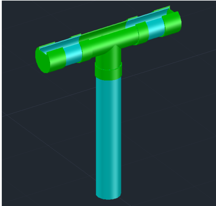
Figure 3: Entrance Tank Overflow Tee AutoCAD drawings
