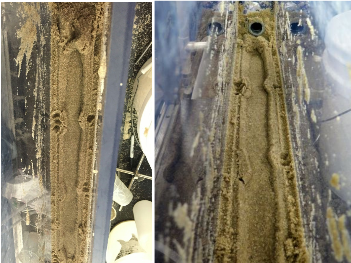
Figure 9: Pictures of the sand exclusion zone and its point of failure.
