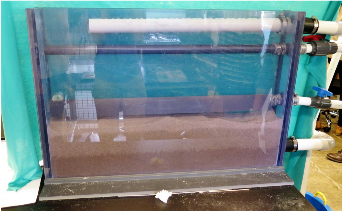
Figure 2: Constructed 10 cm x 86 cm filter apparatus. From top to bottom, the pipes are: backwash outlet, inlet, filtration outlet, inlet. The bottom inlet is within the sand layer.
