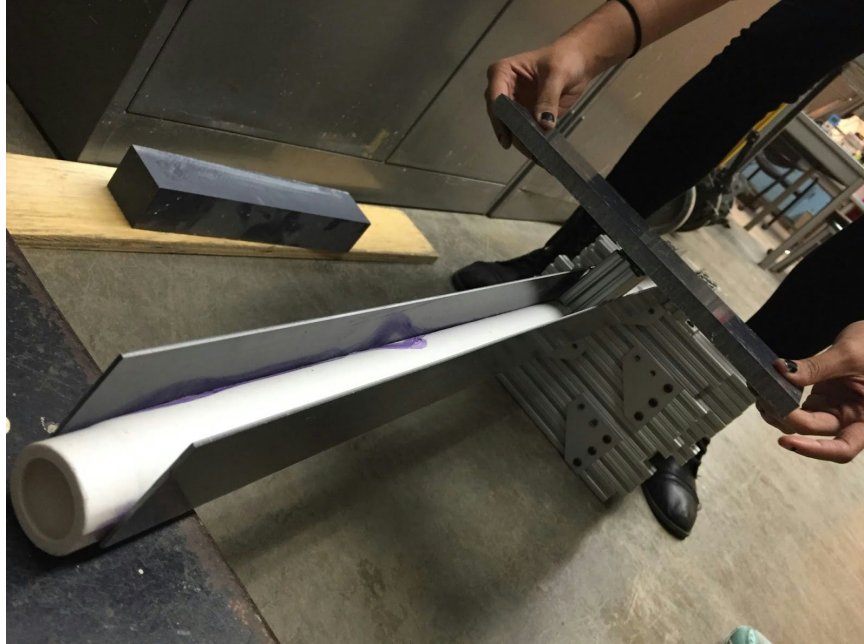
Figure 7: The inlet was placed on an 80x20 support on one side (shown on the right) and on the scale (shown of the left). A force was manually applied to the center of the inlet.
