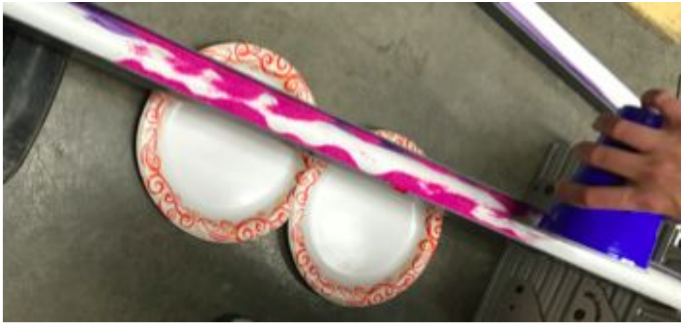
Figure 8: The pink sand leaked when the winged design failed..
