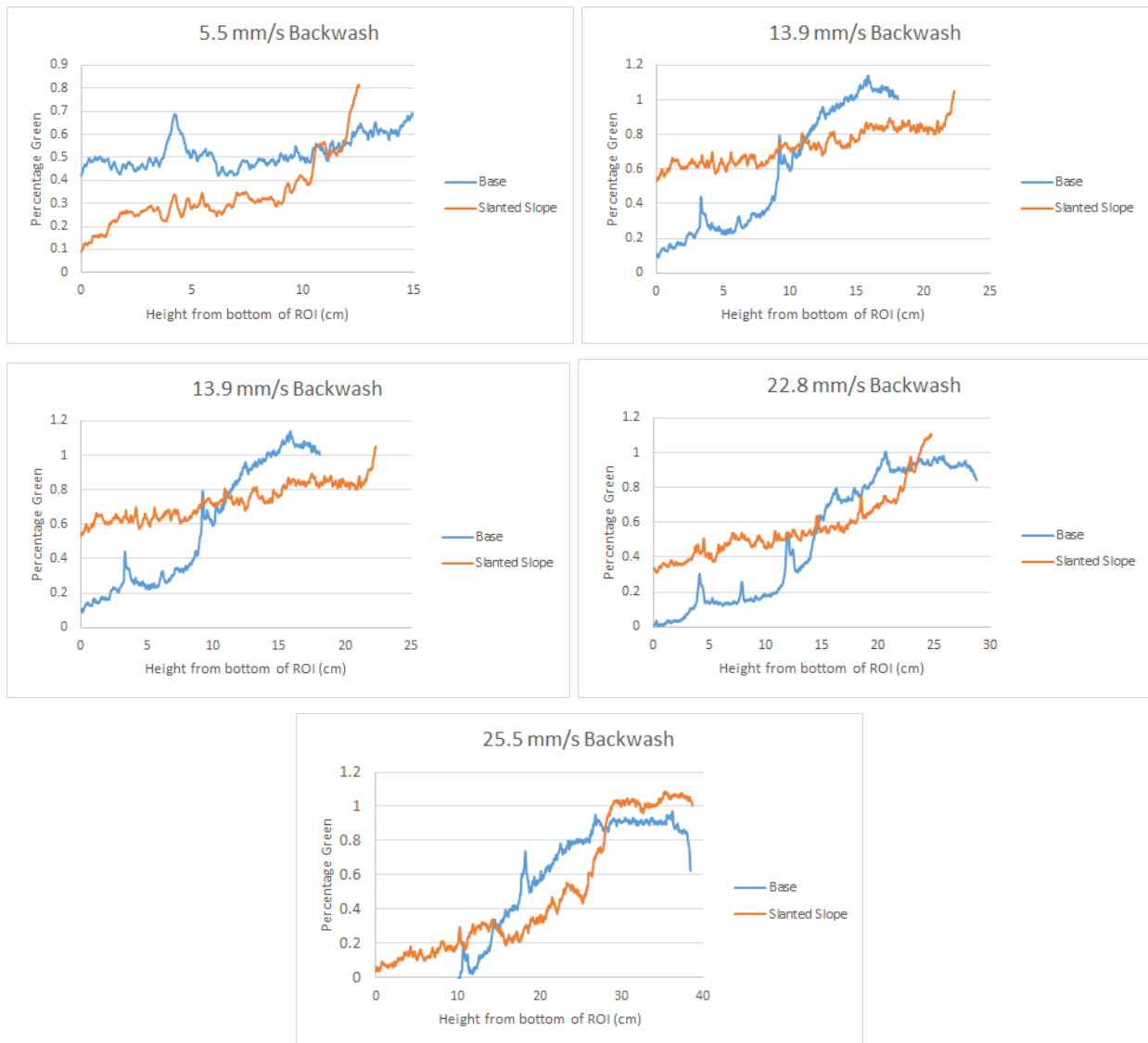
Figure 9: Comparison of the sand segregation with and without the slanted bar, where the base is in blue and slanted slope is in orange. The data is presented with the height from the bottom of ROI (cm) as the independent variable and the percentage of sand that is green as the dependent variable.
