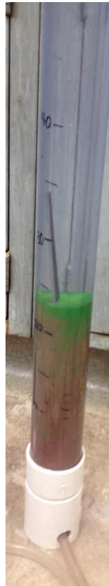
Figure 4: Steel bar placed within the filter to act as a slanted slope
