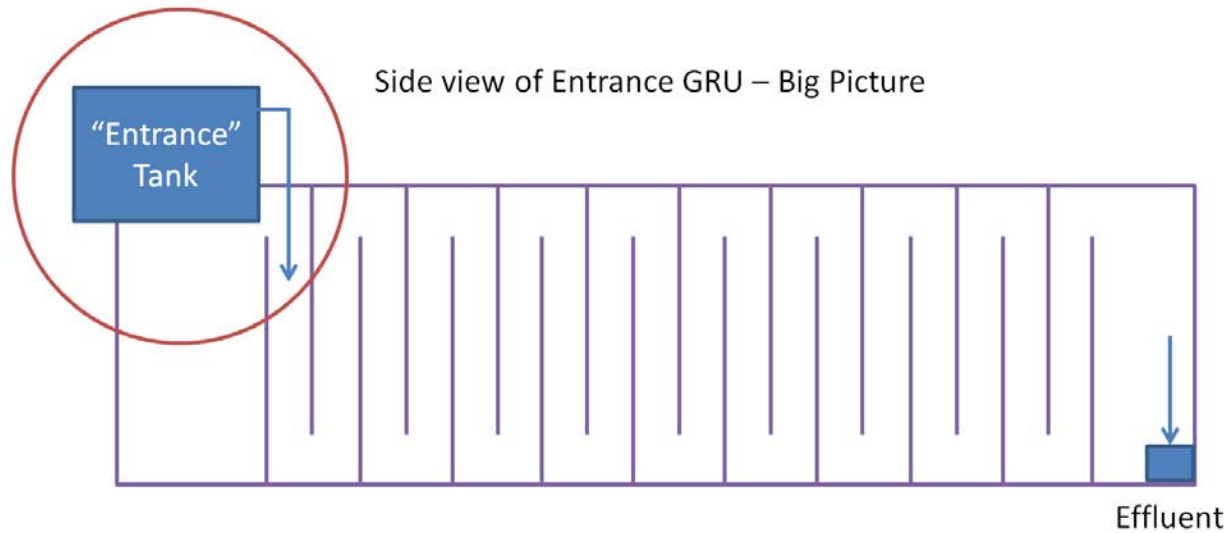
Figure 3.a.ii. The side view of entire flocculator channel, to show placement of entrance tank.
