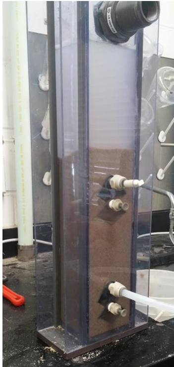
Figure 8: Filter after the bed was filled with sand, and with exclusion zones visible below the inlet and outlet piping
