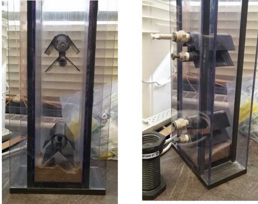
Figure 7: Filter with pipes inserted, before sand has been added to fill the filter bed
