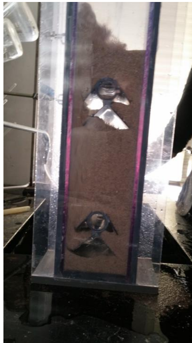
Figure 13: The sand bed only partially fluidized during backwash
