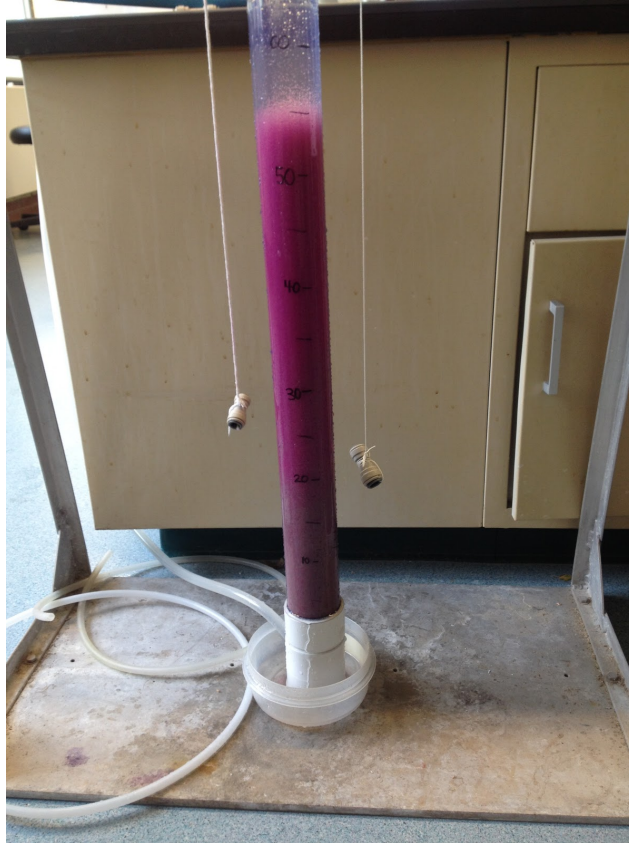
Figure 5: Filter column with two parallel hanging plumbs
