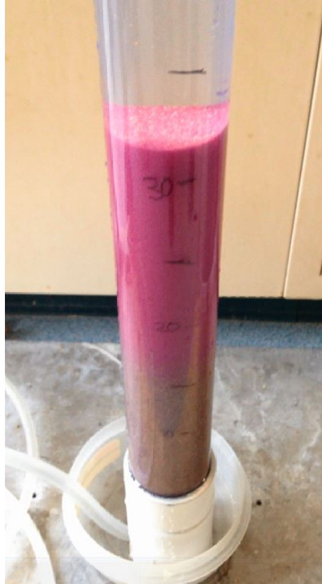
Figure 4: Sand segregation based on sand color distribution
