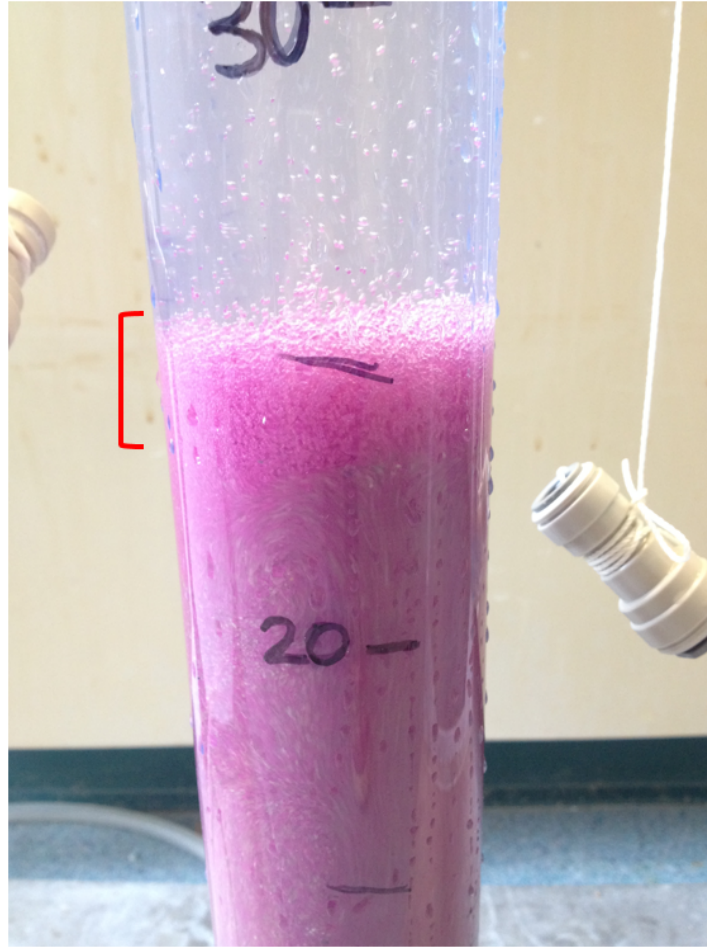
Figure 7: Air bubbles suspending small sand grains
