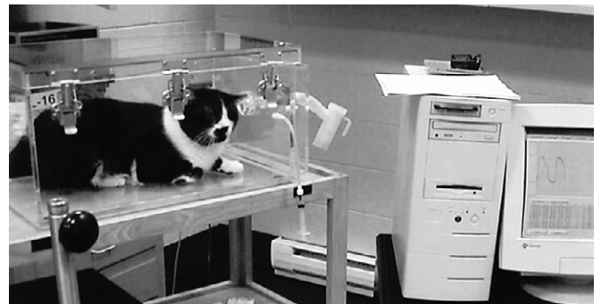
Figure 24-3. Barometric whole-body plethysmography is performed by placing a cat within a plethysmograph. Note that the cat is free to move about and appears to be resting comfortably.
