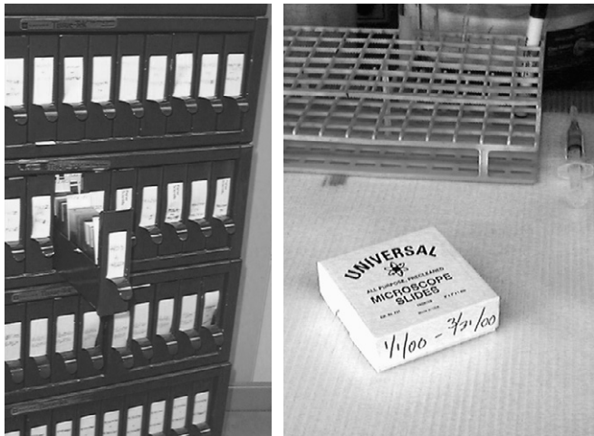
Figure 21-2. Slides can be stored in either file cabinets designed for slides or in empty slide boxes. Labeling can be by accession number or date.
