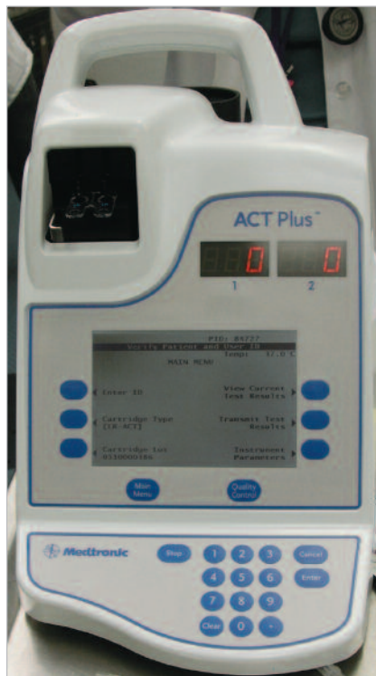
Figure 2. Automated coagulation timer. An accurate determination of coagulation status is critical to prevent clotting within the dialyzer and spontaneous bleeding in the patient.
