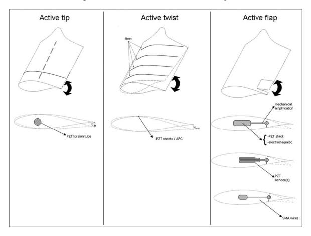
**Figure 6.** Schematics of smart structure concepts.
