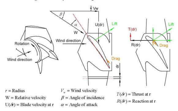
**Figure 9.** Aerodynamic forces generated at a blade element.
