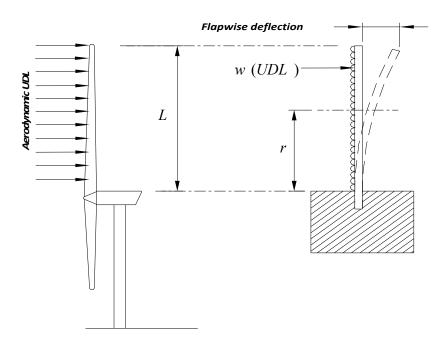
**Figure 11.** Flapwise bending about the axis xx.
