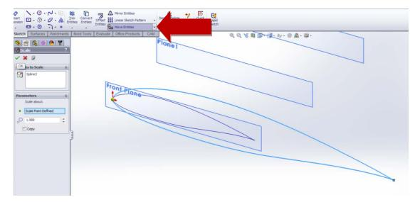
Repeat the process for the next **Plane**. Create a **Sketch** on that **Plane**, use **Convert Entities** to project the **Curve** onto the **Plane**, and use the **Scale** tool to **Scale** the airfoil. Now in the **Sketch Toolbar**, click **Move Entities> Rotate Entities**. Select the **Origin** as the **Rotate Point**. Adjust the angle of the airfoil to position it relative to the first airfoil on the **Front Plane**.
