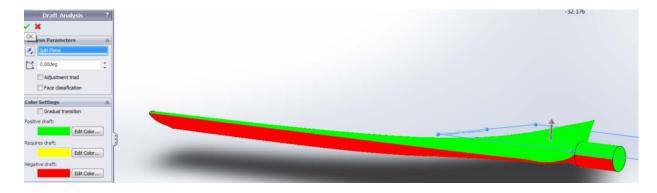
The diameter of the endmill will limit the minimum radius that the CNC router will be able to machine. To allow for the sharp trailing edge of your blade to be machined, the trailing edge of the blade must divide the areas of positive and negative draft. If the blade does not smoothly divide into areas of **Positive** and **Negative Draft** divided by the trailing edge, you will need to adjust the angle of the **Split Plane** so that it does.
