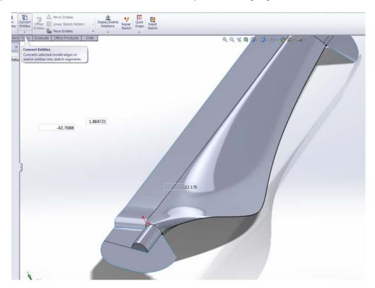
The other two **3D Sketches** were created by drawing **Lines** from the corner of the edge of the adjacent **Parting Surface** to the end point of the **3D Sketch** containing the trailing edge.
