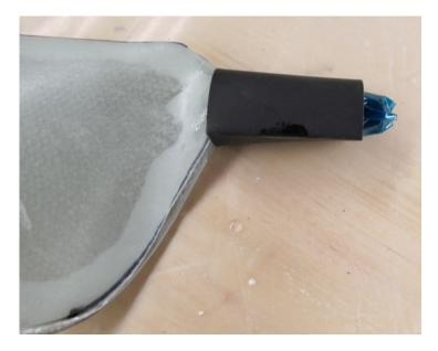
Use a heat gun to shrink the tubing so that it tightly compresses around the blade root. Heat all sides of the tubing so that it shrinks evenly. <u>Do not get epoxy on the heat gun.</u> Wipe off any excess epoxy that has been squeezed out by the heat shrink tube.
