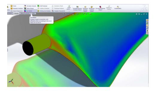
The tip of the blade is still unenclosed. Use the **Filled Surface** tool to create a flat patch across the end of the blade. Use the edge of the tip as the **Patch Boundary**.
