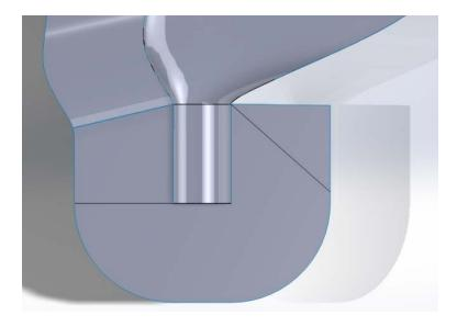
Use the **Delete Face** tool on the **Surfaces Toolbar** to delete the unnecessary face.
