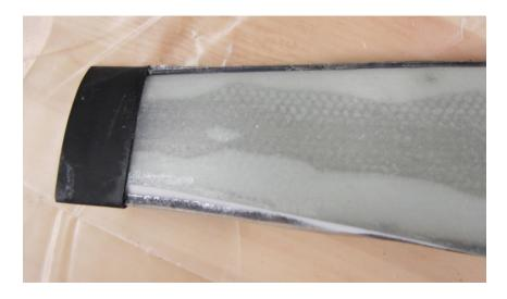
Use a heat gun to shrink the tubing so that it tightly compresses around the blade. Heat all sides of the tubing so that it shrinks evenly. <u>Do not get epoxy on the heat gun.</u> If heat shrink tubing is not being used for the blade tip, use flash tape to tightly tape the blade tip together.
