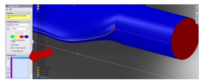
Any flat Faces with zero **Draft** will need to be **Split**. Assuming that your split plane is perpendicular to the ends of your blade, you will need to **Split** both ends.
