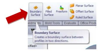
Select the edge of the blade as the **Direction 1 Curve**. Select the two bordering edges of the existing **Parting Surfaces** as the **Direction 2 Curves**. A preview of your **Boundary Surface** should appear. If so, click the check mark.
