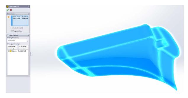
Click **File>Save As** and save the file as a **IGES** (.igs) file. **IGES** is a non-proprietary interchange file format for **CAD** data.
