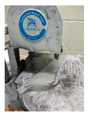
After being trimmed, the blade halves should fit together with minimal gaps.
