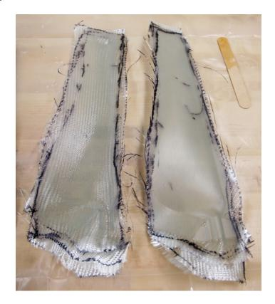
Carefully use a permanent marker to mark the edges of the blade. The edge may be difficult or even impossible to see in some areas, particularly along the trailing edge. It may help to first roughly trim the blade halves and then align the opposing halves so that the opposite side can be used as a reference.
