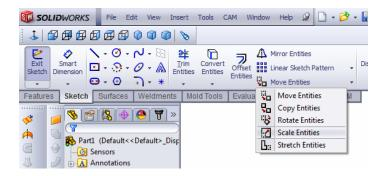
Select the **Origin** as the **Scale Point**. If your original coordinates positioned the leading edge of the airfoil at the **Origin**, this will **Scale** the airfoil around the leading edge. This will appropriately **Scale** the airfoil, assuming that you desire that your blade have a linear leading edge. Adjust the **Scale** to produce the desired airfoil chord length at this point.
