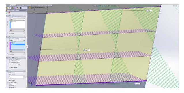
The last step is to **Knit** the **Parting Surfaces**. Do not **Knit** the **Surfaces** of the blade.
