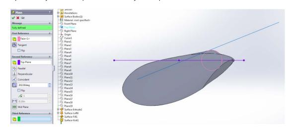
In the **Mold Toolbar**, select **Draft Analysis**. Use the Plane you just created as the **Split Plane**. Set the **Draft Angle** to zero degrees. The blade will be colored to show areas of **Positive** and **Negative Draft**. Because the **Draft Angle** is set to zero, there will be no areas of **Neutral Draft**. Click the checkmark; the coloration will remain.
