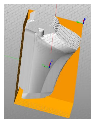
Select **Post-Process Operation** in the **Wizard**. This will output the toolpath as G-Code that can be used by the CNC router. Select **MaxNC** as the **Post Processor**. Click the **Post** button.
