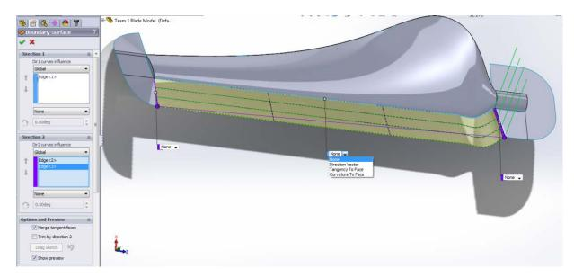
Sections of the **Parting Surface** may be missing. It may be necessary to trim existing sections to allow for a smooth transition. To do so, create a **Sketch** on one of the existing **Planes** to mark where to trim the **Surface**. On the **Mold Toolbar**, select **Split Line**.
