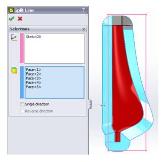
Use the **Delete Face** tool on the **Surfaces Toolbar** to delete the faces that lie outside of the 14x3.9 inch box.
