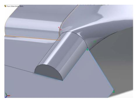
These three **3D Sketches** were then used to define a **Boundary Surface**. The purple **Curvature Comb** is displayed to highlight areas of high curvature. In this case, the **Curvature Comb** indicated a problem area. However, Solidworks was able to produce the **Boundary Surface**.
