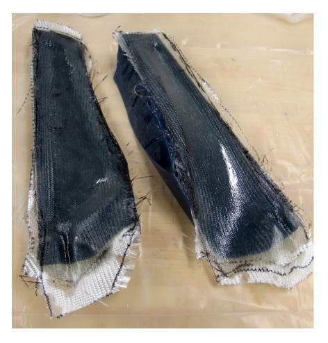
Note: The pieces of fiberglass will stretch. This will likely be particularly apparent when working with the +/-45° pieces. If care is not taken to avoid stretching the pieces, the pieces may stretch until they no longer fully cover the mold.
