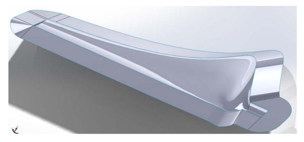
Use the **Knit** tool to **Knit** the **Parting Surfaces** and blade half. If necessary, check the box(es) to close any gaps.
