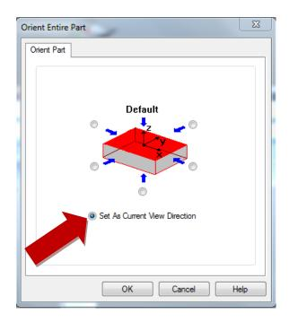
Check that the **Z-Axis** is now normal to the prior location of the **C-Plane**. Because this will be a female mold, the **Z-Axis** should be pointing towards what will become the interior of the blade. If the **Z-Axis** is inverted, again click **Transform>Part Orient...** and, this time, select the arrow facing upwards before clicking **OK**. The **Z-Axis** should now be facing the correct direction.
