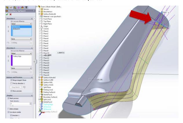
From a distance, the **Boundary Surface** appeared acceptable, however upon closer inspection it became apparent that there was a small wrinkle.
