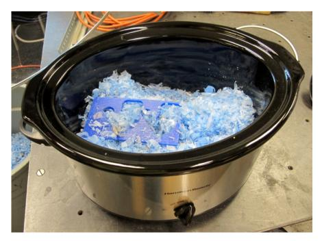
Note: Machining wax has a melting temperature of around 226° F. To fully melt the wax, it will need to be heated to 270-290° F. If it is heated above 300° F it may begin to burn. These numbers are given as a reference; you should not need to measure the temperature of the wax.
