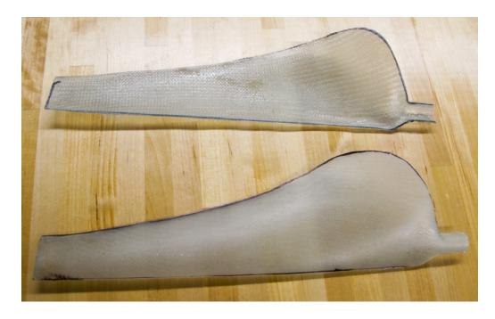
The pieces will need to be sanded to ensure adhesion and improve the fit of the pieces. Use 100 grit or rougher sandpaper. Rough up the interior sides of the pieces along the edges of the piece. Rough up both the interior and exterior sides of the blade root areas. It may be helpful to bevel the edges of the pieces to allow the pieces to fit more closely together.
