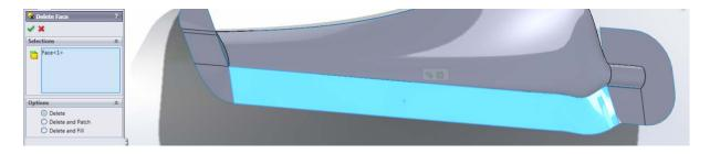
Replace the face using a **Boundary Surface**. Boundary Surfaces are defined by two or more edges or **Sketches** that form the boundary of the **Surface**.
