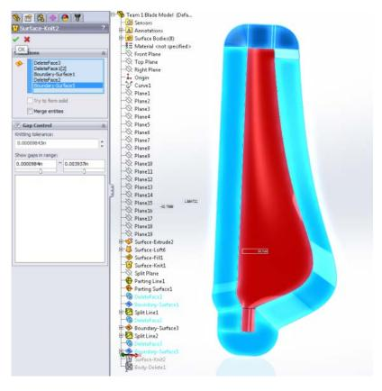
In this case, it is not necessary to model the rest of the molds. Only the mold cavities and **Parting Surfaces** will be machined.
