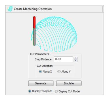
A toolpath will be displayed with blue lines. These should be orientated so as to run along the length of the blade. The **Engage** and **Retract Feeds** will be shown in red and yellow.
