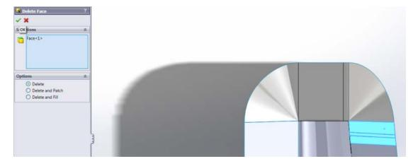
Upon further inspection, it became apparent that the source of the problems was that the **Parting Line** zigzagged slightly.
