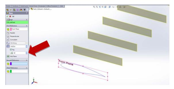
Create a **Sketch** on the **Front Plane**. Use the **Convert Entities** tool to project the airfoil **Curve** onto the **Front Plane**.
