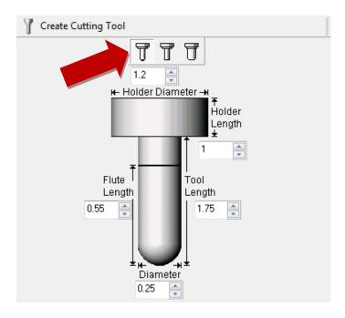
Select **Set Cutting Feeds and Speeds** in the **Wizard**. Set the **Spindle Speed** to 8,000 RPM. Set the **Cut Feed** to 1000 in/min. Set the **Engage Feed**, and **Retract Feed** to 100 in/min.
