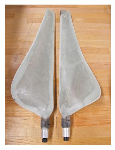
Apply Loctite thread-locking compound to half of a 1 inch long 1/4-20 threaded steel stud. Screw the end of the stud that has been coated with Loctite into the aluminum blade root until 1/2 inch of the stud remains protruding. Allow the Loctite to harden. The blades are now complete and ready for testing.
