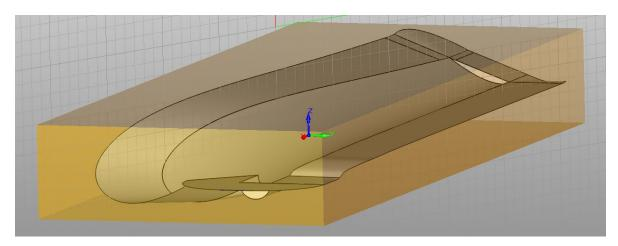
Click **Set Machine Zero** in the **Wizard**. The **Machine Zero** is the point that the CNC router will consider to be (0,0,0,). Select **Set to Stock Box**. The **Stock Box** will appear in the **Viewpoint**. A second set of larger axes will be visible. These represent the **Machine Zero**. Under **Zero Face**, select **Highest Z**. This will locate the **Machine Zero** on the top face of the Stock Box.
