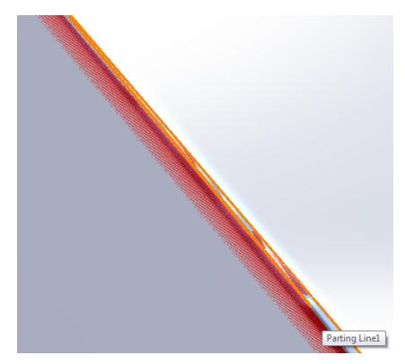
As a workaround, **3D Sketch** was created and a **Spline** was closely fit to the **Parting Line** while omitting the zigzag.
