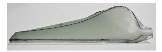
Use a diamond grit band saw to trim the blade halves. Ensure that the water reservoir has been partly filled before using the saw. Remember that while you can always trim more material, including after the blade has been assembled, you cannot replace material that you have trimmed. Err on the side of caution when choosing where to cut. Wipe off the saw when finished.
