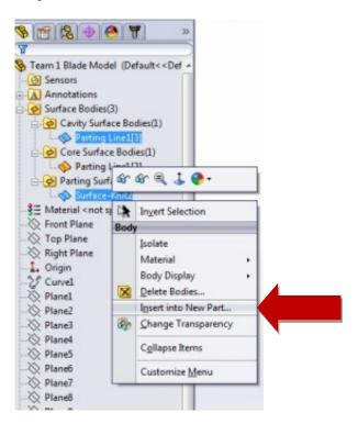
The **Save As** dialogue will open. Name your mold half as either the front (upwind) or rear (downwind) mold half and save it. The file should include the **Parting Surfaces** and only one half of the blade. It will be zero-thickness.
