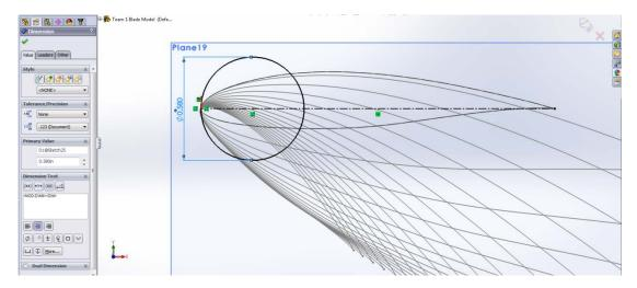
You may find it helpful to define **Construction Geometry** to position the circle (as shown below). You can always go back and adjust the position of this circle later.
