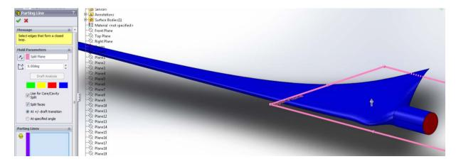
Select an appropriate edge as a **Parting Line**. Solidworks will attempt to identify the next contiguous segment. Solidwork's guess will be highlighted yellow and a red arrow will point toward it. If the guess is incorrect, click the red arrow to switch between the possible edges until the proper edge is identified. Then, select that edge.
