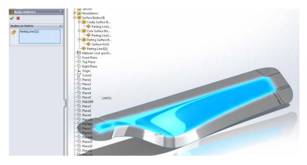
The next step is to create two new files containing each half of the mold. Select both the **Parting Surface Bodies** and the **Cavity Surface Bodies**. Right click and select **Insert into New Part...**
