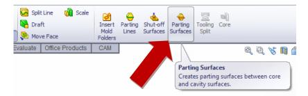
Select **Perpendicular to Pull**. Select the your **Parting Line** as the **Parting Line**. Set the length of the **Parting Surface** as 1 inch. Check the boxes next to **Knit all Surfaces** and **Show Preview**. It is likely that Solidworks will be
