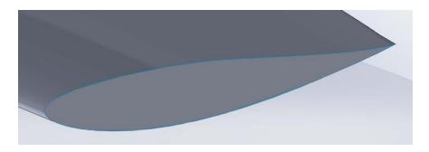
The **Knit** tool is used to merge **Surfaces**. This tool is capable of automatically identifying and "knitting" together small gaps. To use it, click the **Knit Surface** tool on **Surfaces Toolbar** and then select all three **Surfaces** you have created. There should be no need to adjust the **Knitting Tolerance** or other settings. If any larger gaps are identified, they will appear under **Gap Control**. If this occurs, check the box(es) to close these gaps.
