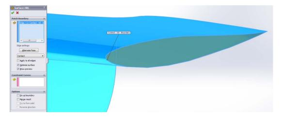
A shown below, the a blue line will be displayed along the edge of the **Fill**. The same is true where the **Extrude** meets the **Loft**. Blue lines signify edges where **Surfaces** are not actually connected. Were you to zoom in close enough, you would begin to see small gaps between the surfaces along these lines.
