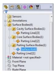
You likely will a redundant **Surface Body** consisting of the entire blade. This is no longer necessary, so right click it and select **Delete Body...** to delete it.
