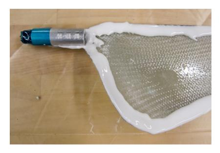
Press the two halves of the blade together. If there are any areas where the gap between the two halves have not been filled with epoxy, add epoxy to fill the gap. Wipe off any excess epoxy with paper towels. If heat shrink tube is being used to secure the blade tip, slide a 1/2 inch. section of heat shrink tube over the tip of the blade.
