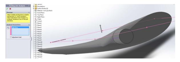
Click the checkmark. The **Parting Lines** will remain visible until the **Parting Line Analysis** button is clicked again. Next, click the **Parting Lines** button to create the parting lines.
