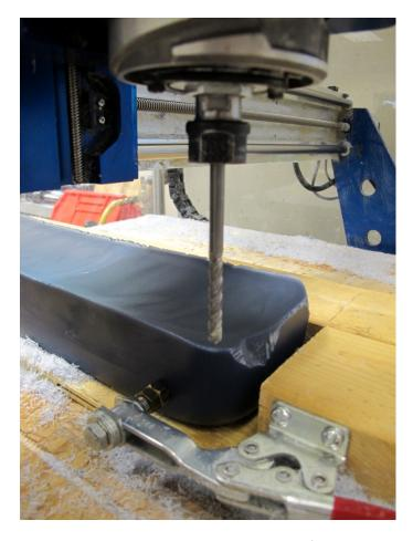
Turn on the router spindle using the black switch located on top of the router. Shut the Plexiglas door. Using the **Jog** commands, lower the router so that the tip of the end mill plunges roughly 1/8 inch. into the wax block. This will ensure that the machined surfaces will not extend beyond the top surface of the wax block. Open the Plexiglas door and shut off the router spindle.
