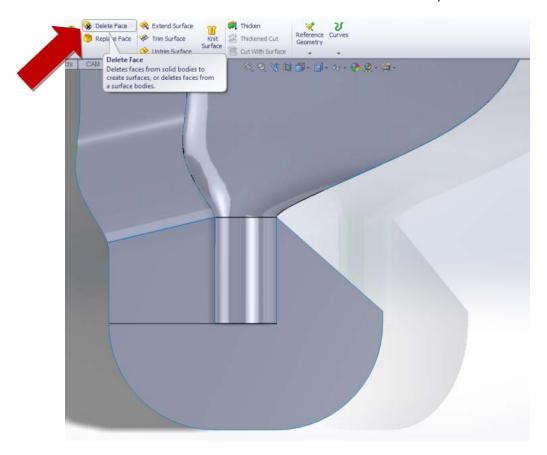
The next step is to attempt to use a **Boundary Surface** to create the missing section of the **Parting Surface**. If you ever attempt to create a **Boundary Surface** and find that it is twisted, right click one of the selected Curves and click **Flip Connectors** to untwist the surface.
