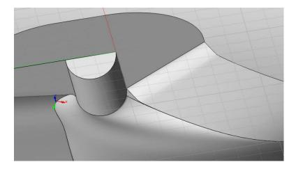
If you need to adjust the **C-Plane**, you can also use the other **C-Plane** tools such as **C-Plane>Set by 3 Pts**. Once the **C-Plane** has been appropriately positioned, right click on the **Viewport** (without selecting a part geometry) and click **Align to C-Plane**.
