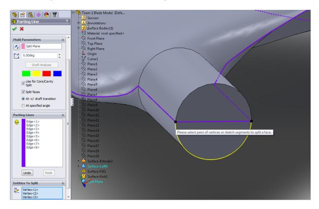
Once you have closed the loop of Parting Line segments, click the checkmark to create the Parting Lines.
