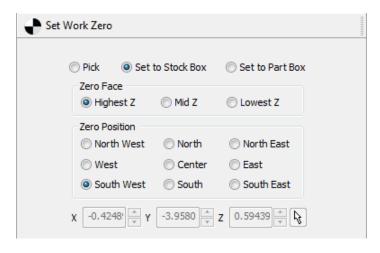
Set the **Zero Position** so that the **Machine Zero** is located on the **South West** corner.
