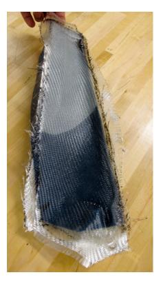
The outer surface of the blade (the surface that was against the mold) should be smooth and largely free of imperfections. The pieces will still need to be trimmed.
