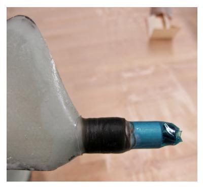
The edges of the blades will need to be sanded to round the edges and remove excess material. Use 60 grit sandpaper to shape the edges. Smooth the blade root area, but do not sand completely through the basalt.
