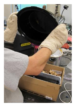
Cover the loaf pan. Leave it to cool for 12 hours. Once it has cooled, you can remove the wax from the loaf pan. Machining wax shrinks approximately 7% when cooling. As a result, it should be relatively easy to remove from the pan.
