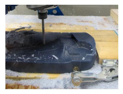
Repeat the process for the second mold. When complete, shut off the router using the red switch on the control box. Close **Maxpath** by returning to the **Main Menu** and pressing **ESC** followed by **Y**. Shut down the computer.
