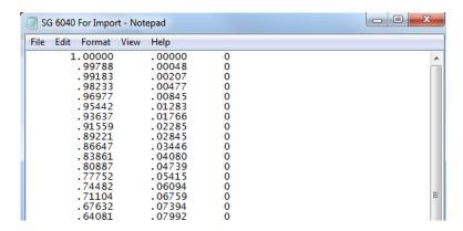
Once you have created the necessary .txt file of coordinates, create a new part in Solidworks and click **Insert>Curve>Curve Through XYZ Points...** to import the coordinates.
