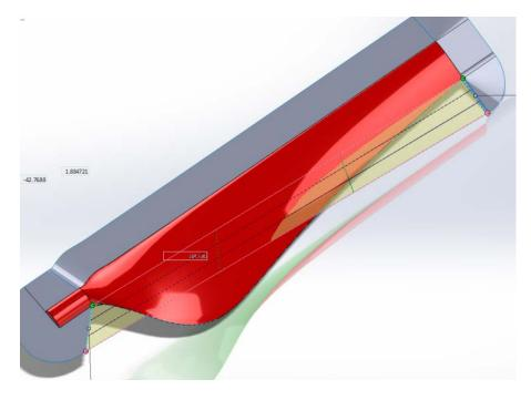
To solve this, three separate **3D Sketches** were created to manually define the three edges of the boundary surface. The **Convert Entities** tool was used to import the trailing edge of the blade into one **3D Sketch**.
