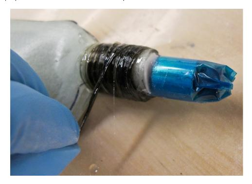
Slide a 1.5 inch long section of heat shrink tube over the blade root.
