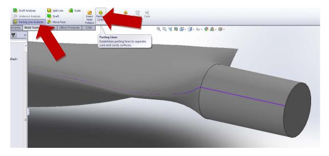
Select your split plane as the **Direction of Pull**. Set the **Draft Angle** to zero and then click **Draft Analysis**. Check the boxes for **Use For Core/Cavity Split** and **Split Faces**. Select **At +/- Draft Transition**.
