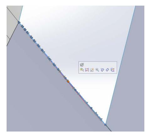
This **3D Sketch**, along with the edges of the existing **Parting Surface**, was used to create a **Boundary Surface** to fill the gap. This left a miniscule gap between the blade and the **Parting Surface**, however the size of this gap was negligible.
