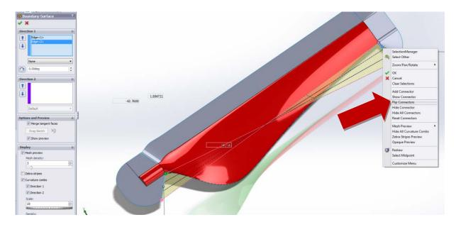
In this case, any attempt to select the trailing edge of the blade resulted in Solidworks crashing. The ends of the edges used to define a boundary surface must meet. In this case, miniscule gaps existed. This is a common reason why boundary surfaces fail.
