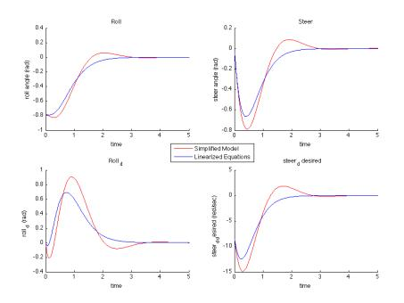
Figure 2: Comparison of the Linearized Equations and the Point Mass Bicycle Equations
