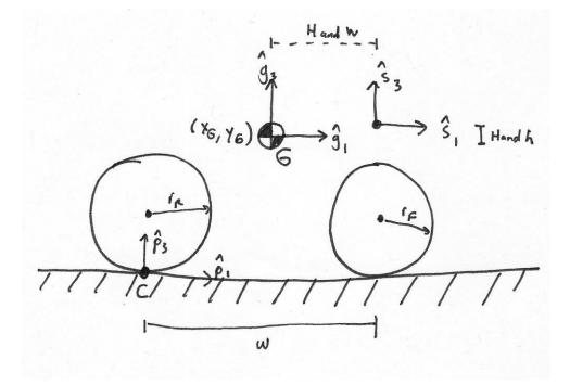
Figure 13: Bicycle Parameters and Frames
