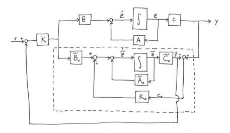
Figure 7: Observer Controller For Reference Tracking Block Diagram
