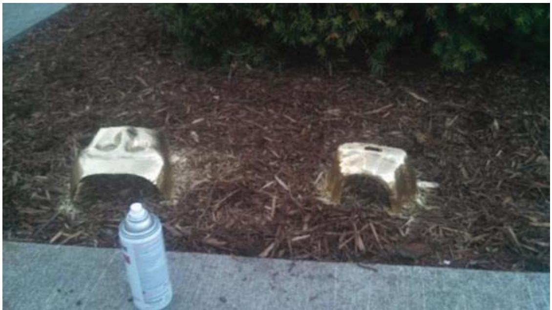
Figure 105: Face parts spray painted outdoors to allow for proper ventilation
