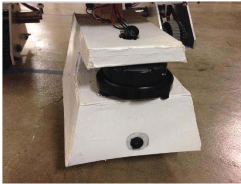
Figure 33: Ultrasonic rangefinder s encased the LIDAR foot
