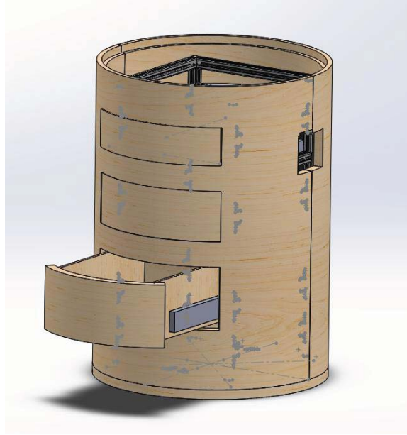
Figure 43: Pull Out Drawer Design and drawer slides within chassis
