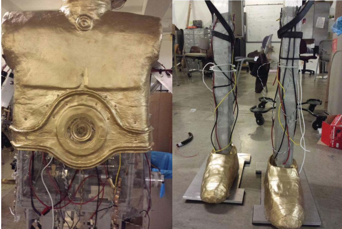
Figure 108: Electrical wire mesh cover on the abdomen and leg
