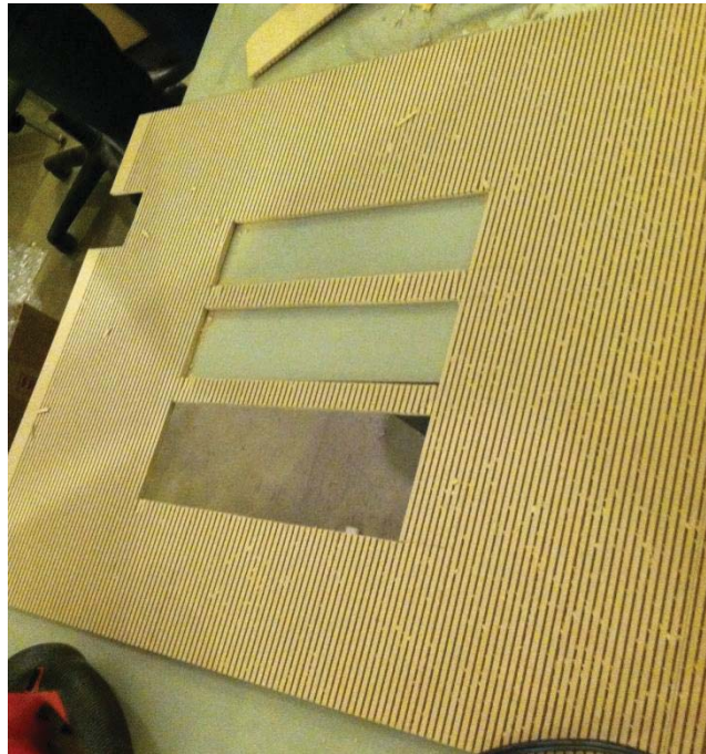
Figure 30: Kerfed wood with rectangular cut-outs
