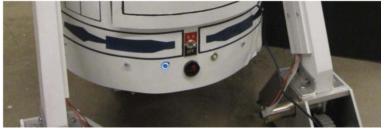
Figure 36: Power and other buttons on R2
