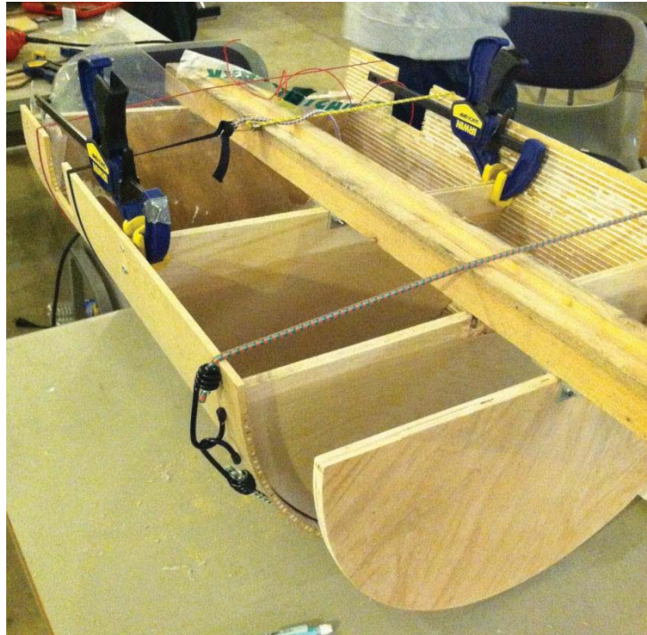
Figure 29: Kerfed wood on shaper
