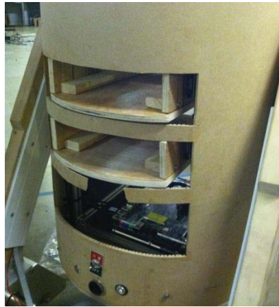
Figure 31: Curved shell on drawer-side of R2
