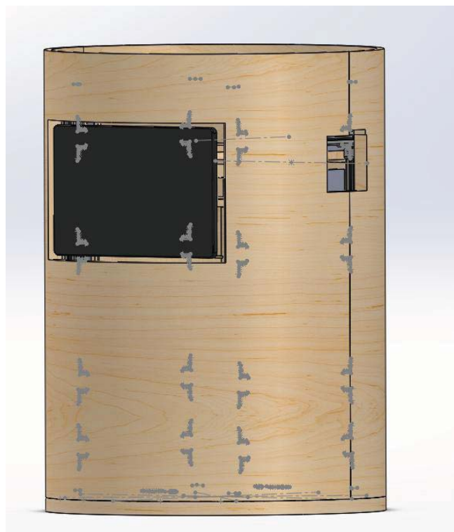
Figure 42: Visible Tablet mounted flush with chassis shell
