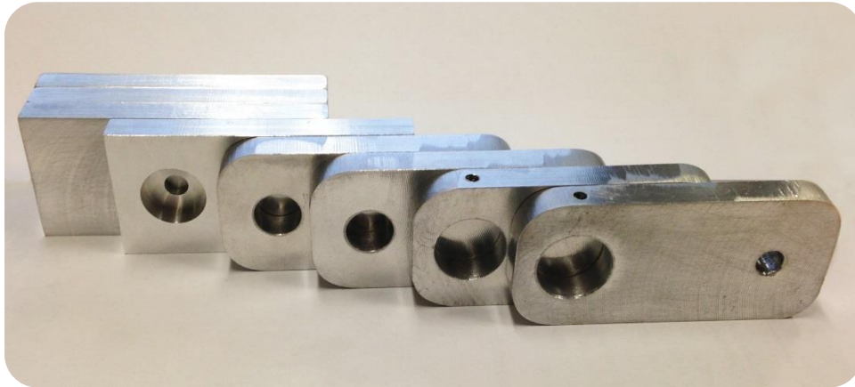
Figure 21: Cranks in Various Machining Stages
