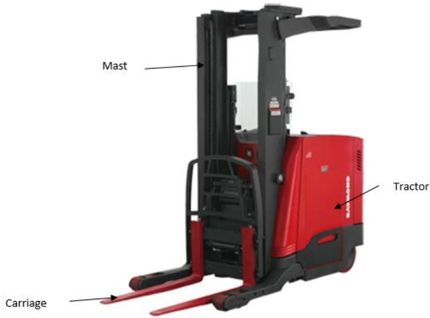
Figure 1: Physical image of Raymond’s reach truck with key components of the model identified
