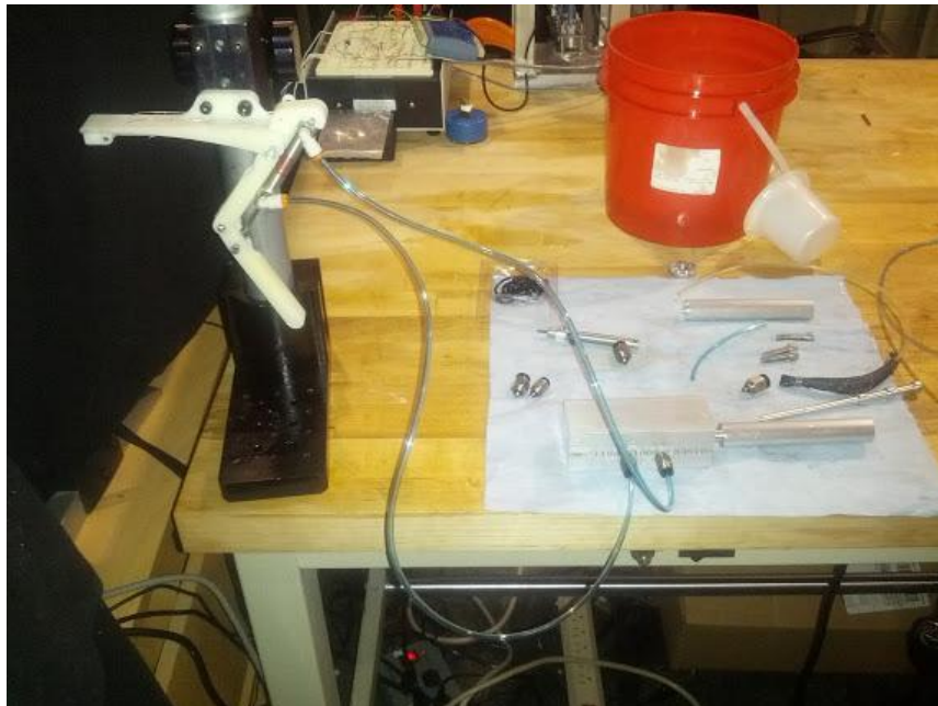
Figure 4: Linear dangle valve prototype with small-scale dangle test leg.
