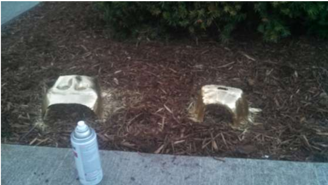
Figure 105: Face parts spray painted outdoors to allow for proper ventilation
