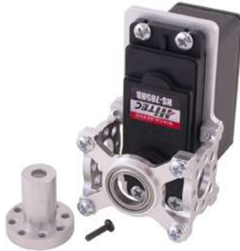
Figure 21: Right wrist servo connector
