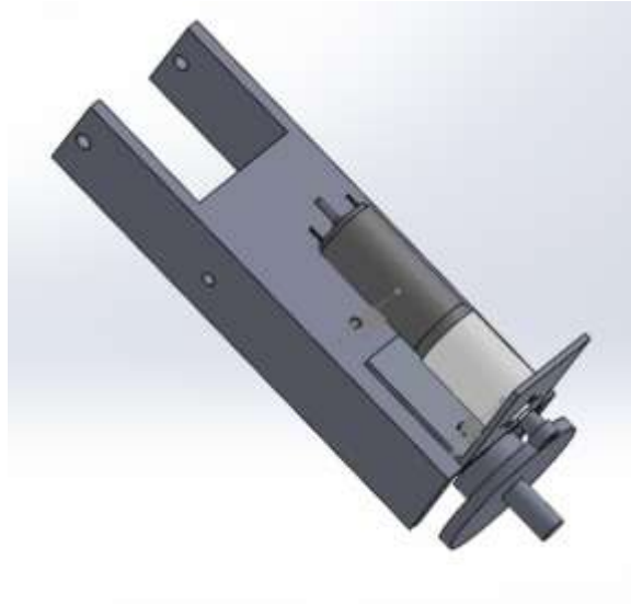
Figure 49: Twist motion, highlighting the 3:1 external gear ratio
