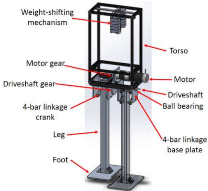
Figure 89: Annotated Four-Bar Linkage Walking Mechanism
