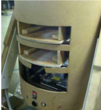
Figure 31: Curved shell on drawer-side of R2
