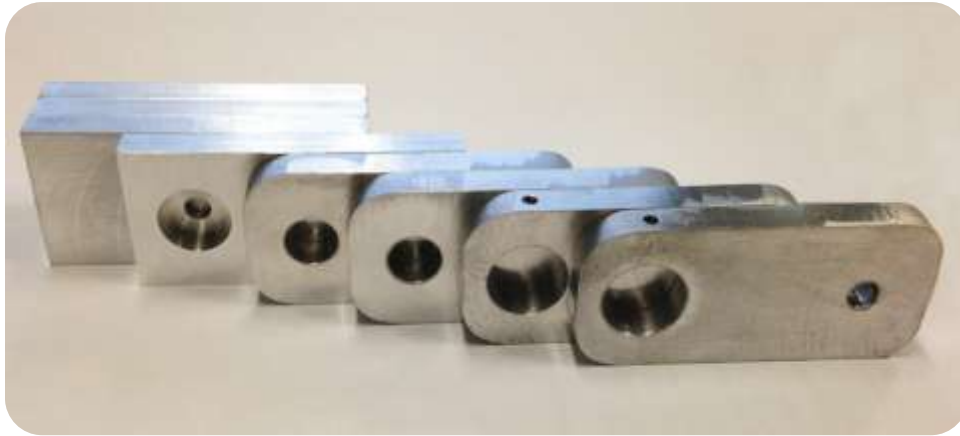
Figure 95: Cranks in Various Machining Stages
