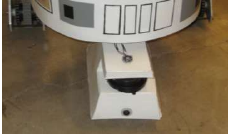
Figure 55: R2's LIDAR foot
