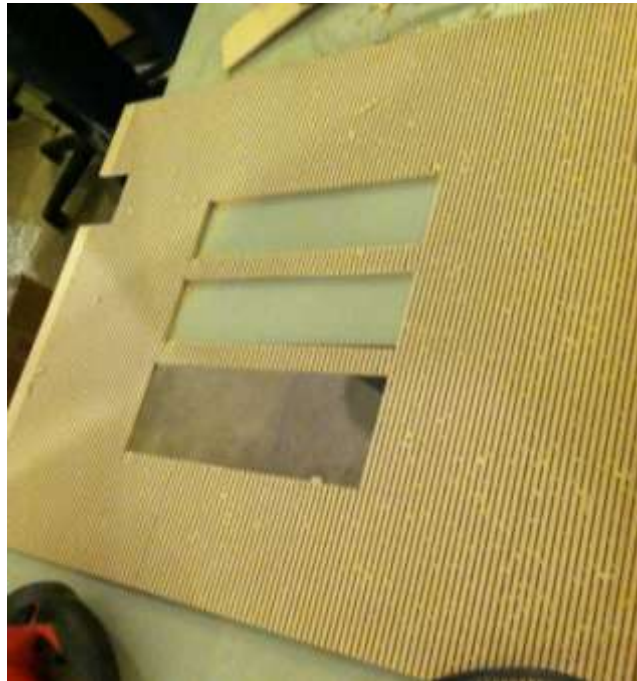
Figure 30: Kerfed wood with rectangular cut-outs
