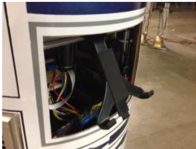
Figure 35: Tablet Mount on Chassis
