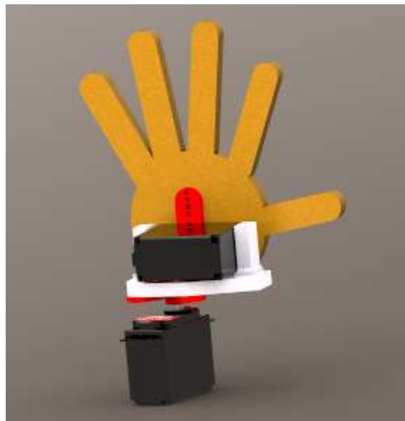
Figure 20: New orientation of servos. The photo is oriented so that the palm of his hand is visible. The bottom servo allows for the twisting motion and the top allows for the right and left motion.
