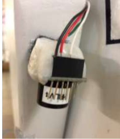
Figure 32: Ultrasonic rangefinder encased in moldable plastic and mounted onto R2's leg
