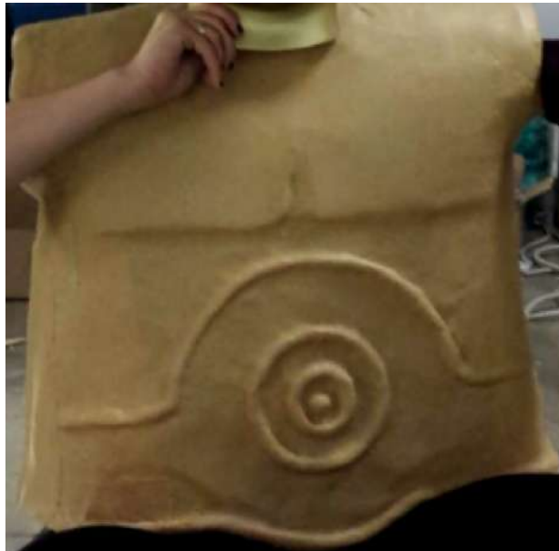
Figure 103: Cooled, formed Worbla sheet
