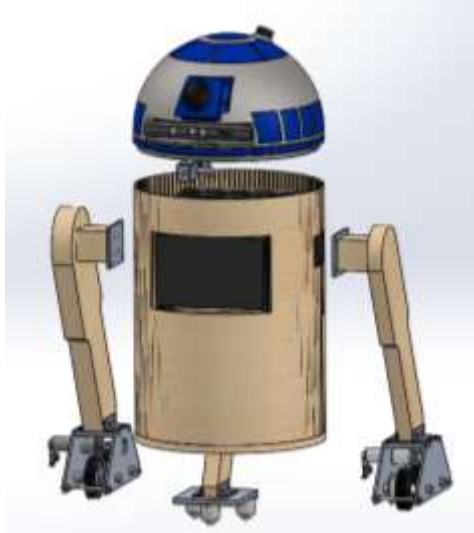
Figure 51: Chassis Integration with head and legs
