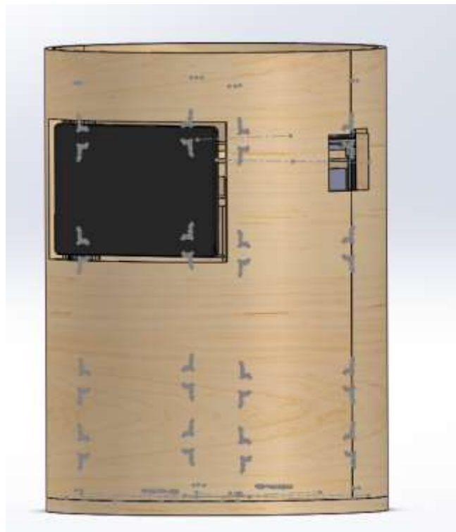
Figure 42: Visible Tablet mounted flush with chassis shell
