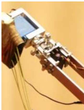
Figure 22: New way to connect servos in right wrist.
