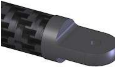
Figure 14: Carbon fiber tube end - Female
