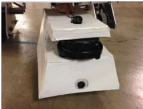
Figure 33: Ultrasonic rangefinder s encased the LIDAR foot
